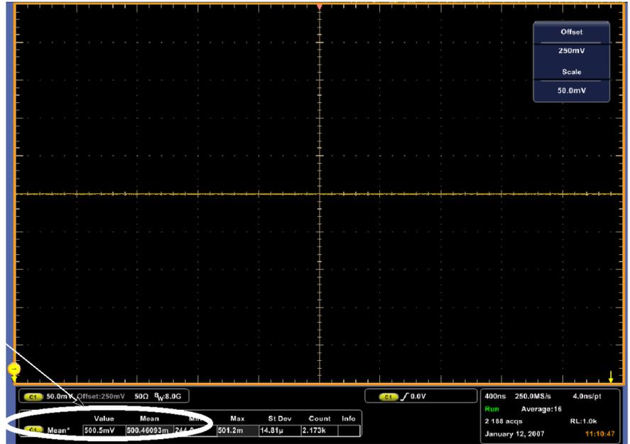
Figure 19: Measurement of offset accuracy
