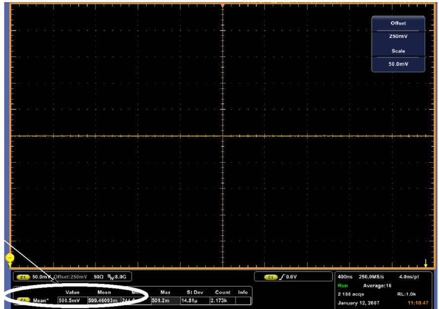
Figure 17: Measurement of offset accuracy
