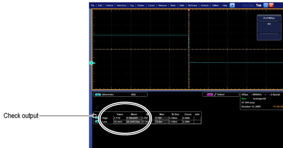
Figure 36: Measurement of trigger out limits
