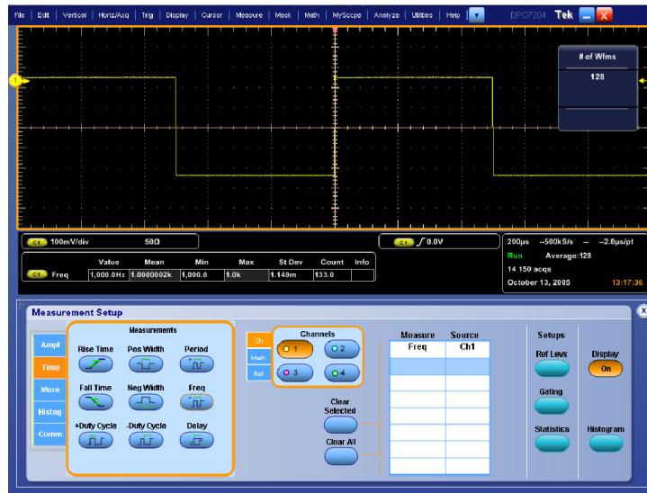
Figure 38: Measurement of probe compensator frequency
