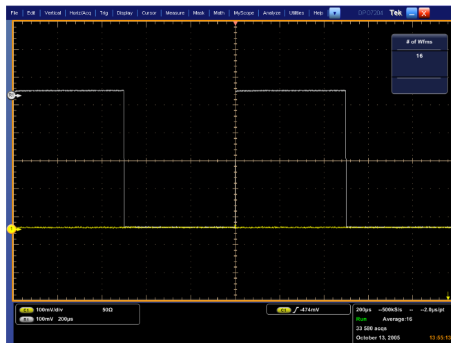
Figure 40: Measurement of probe compensator amplitude
