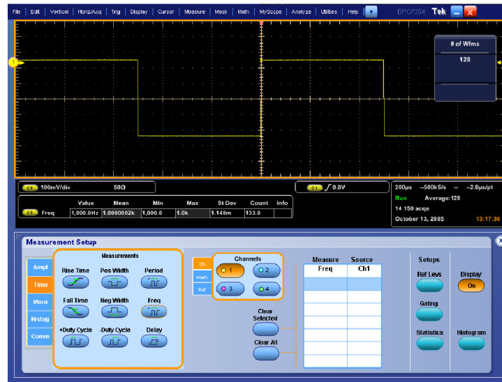
Figure 33: Measurement of fast edge frequency
