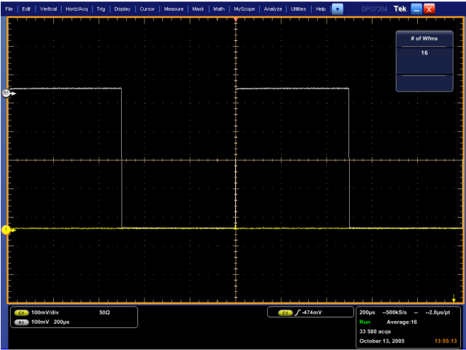
Figure 35: Measurement of fast edge amplitude
