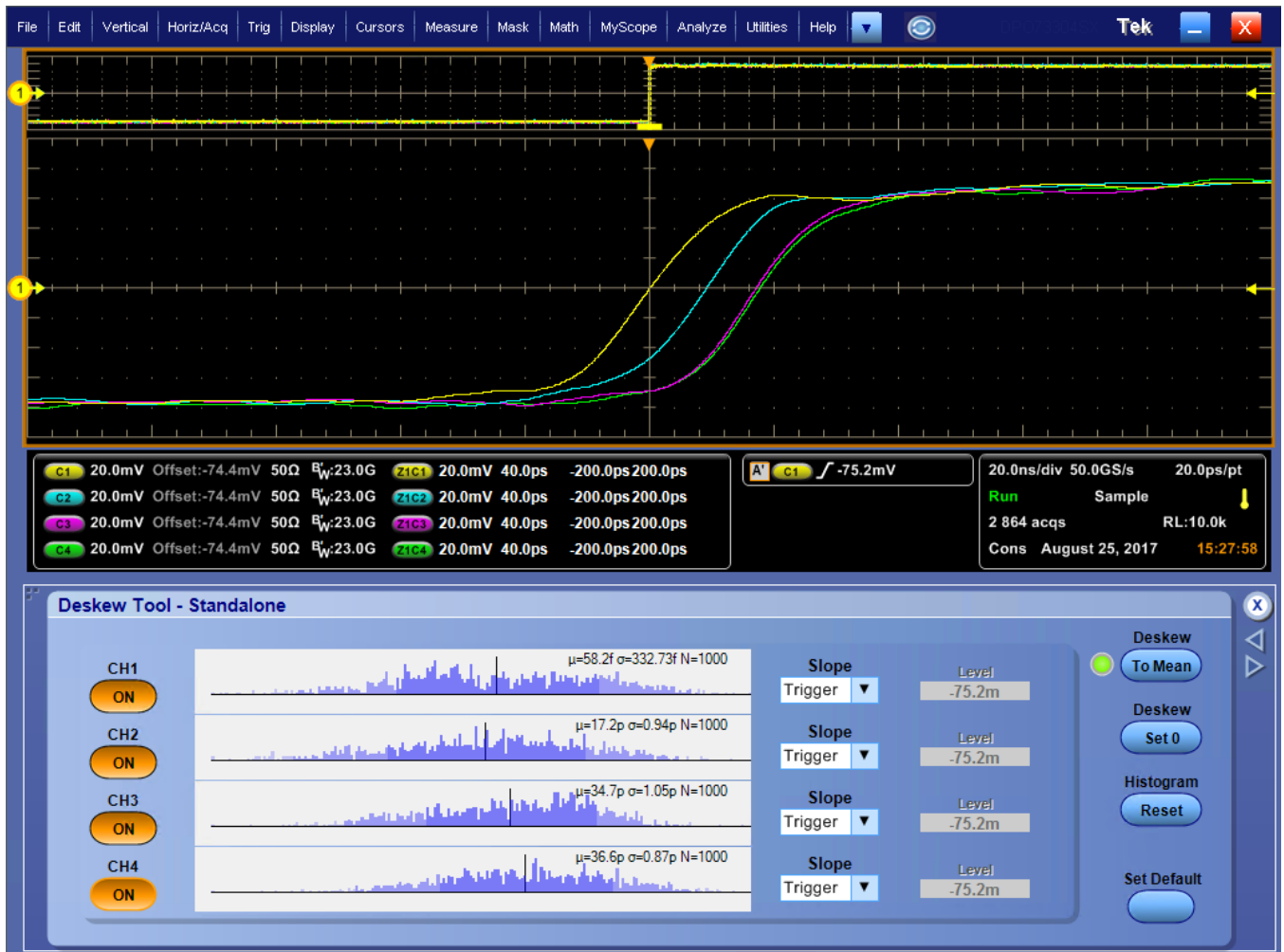
Figure 7: Fast edge signals before deskew
