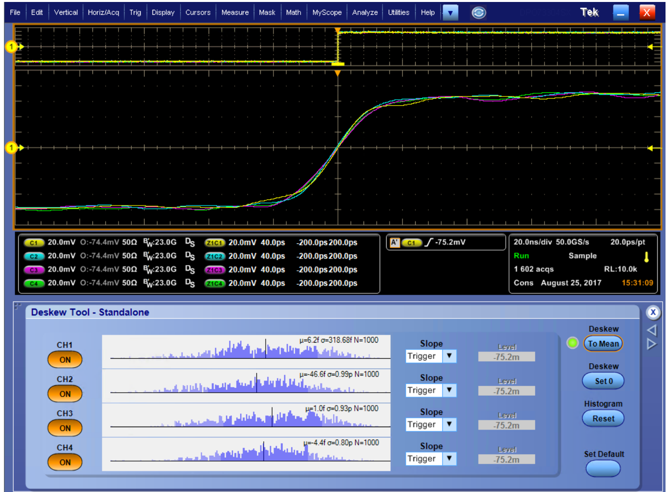
Figure 8: Fast edge signals after deskew
