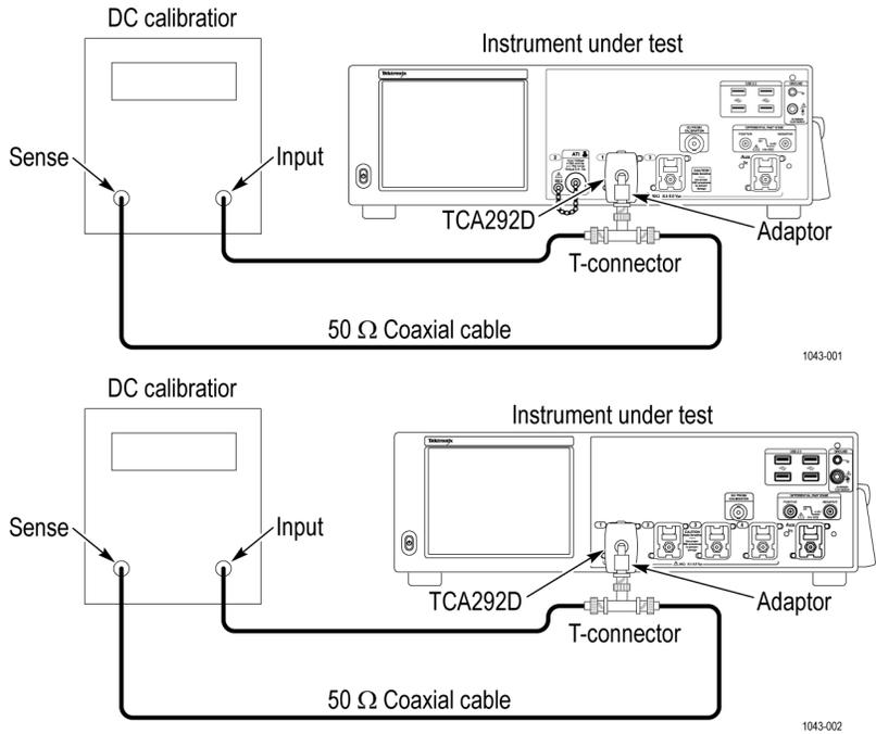
Figure 34: Fast edge output second test hookup
