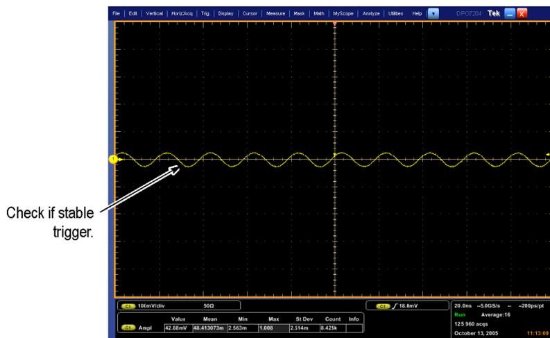
Figure 31: Measurement of trigger sensitivity - 50 MHz results shown
