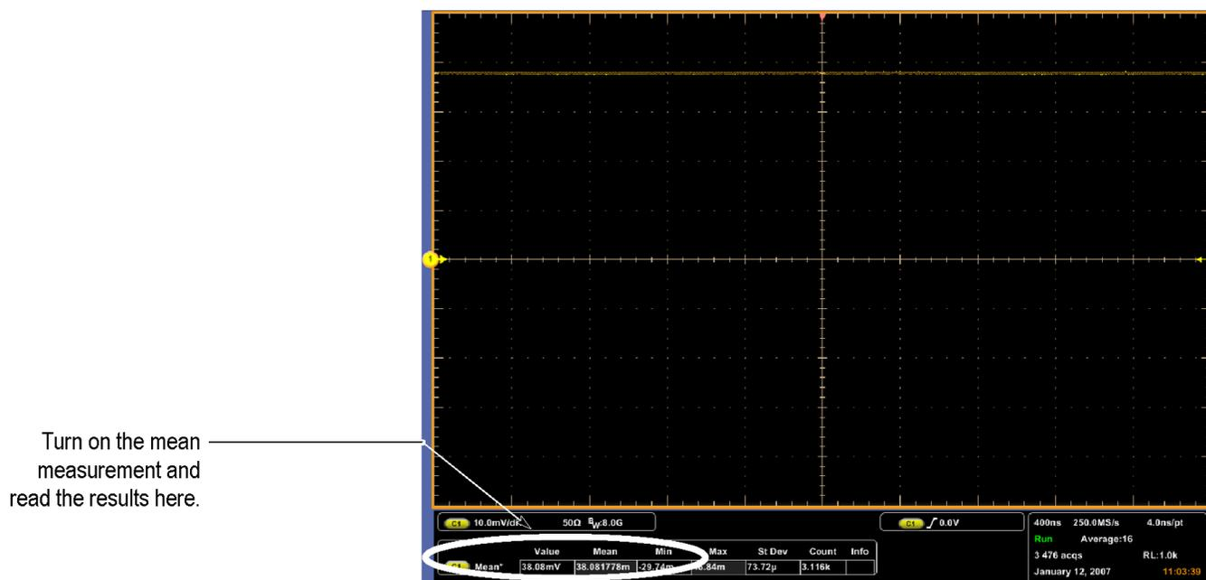
Figure 11: Measurement of DC gain accuracy
