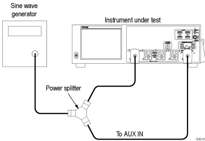
Figure 30: Sensitivity, edge trigger, DC coupled test hookup
