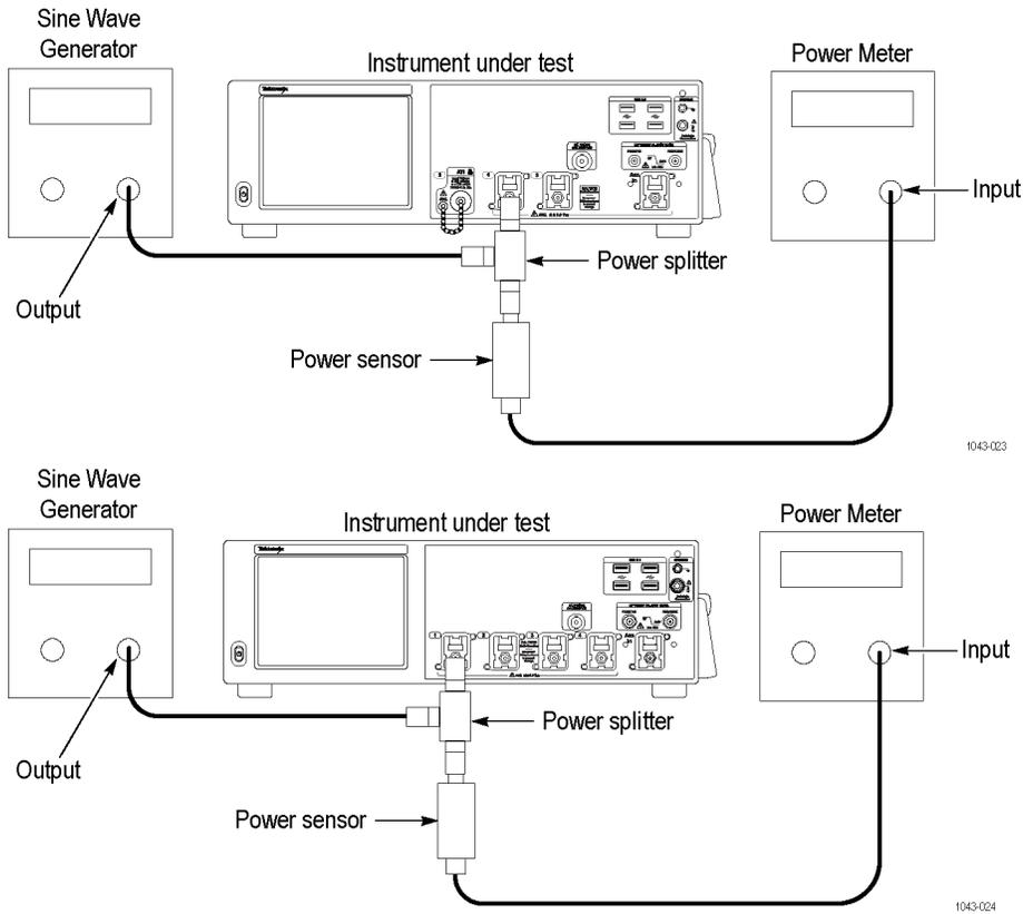
Figure 36: Sine wave generator leveling equipment setup
