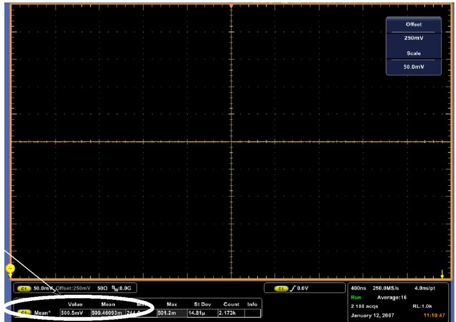
Figure 15: Measurement of offset accuracy
