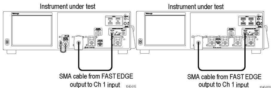
Figure 32: Fast edge output initial test hookup
