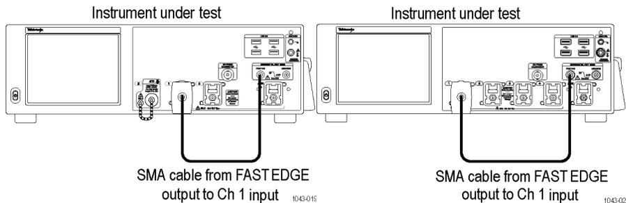
Figure 5: Setup for the file system test
