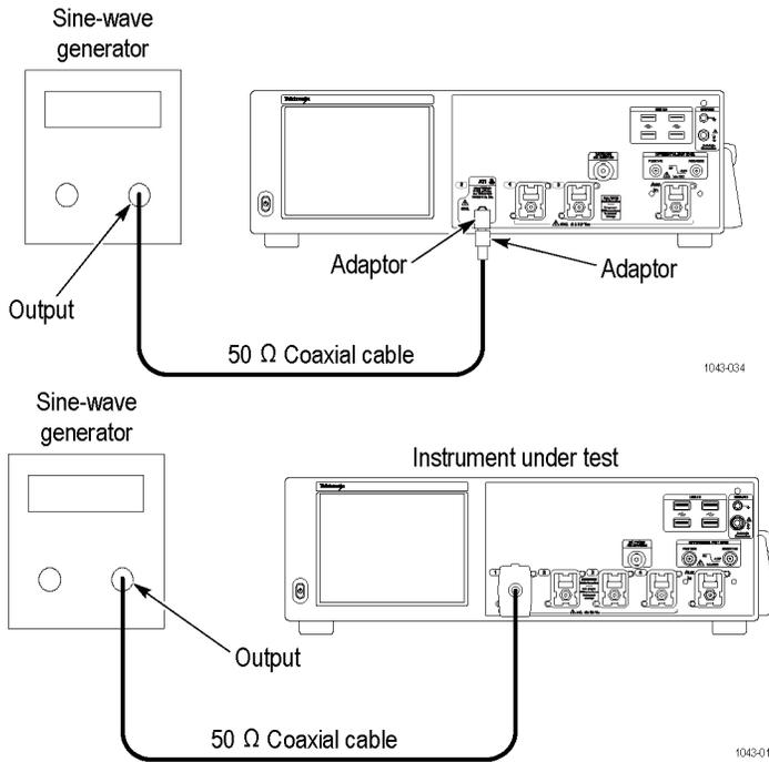
Figure 27: Delta time accuracy test hookup
