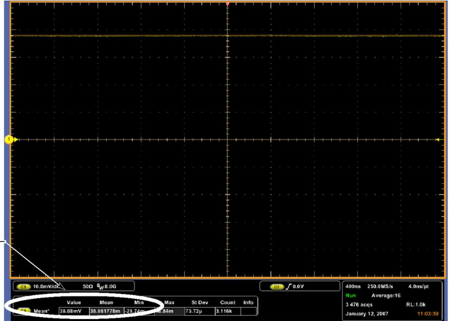
Figure 13: Measurement of DC gain accuracy
