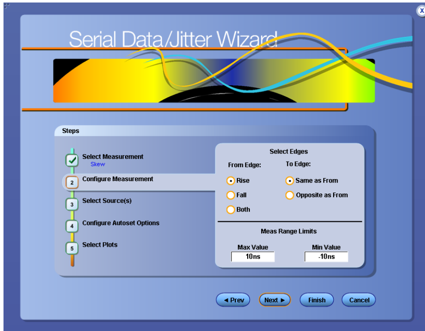
Figure 92: Configure measurement-Skew
