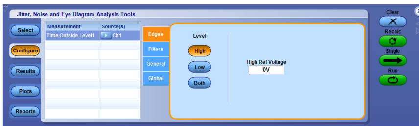
Figure 75: Configuring edges for time outside level
