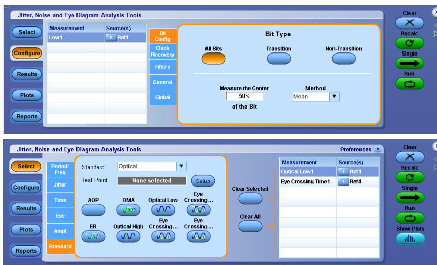
Figure 49: Bit config for amplitude measurements
