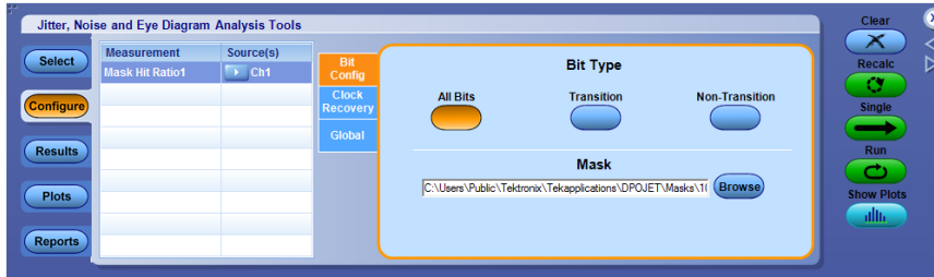
Figure 47: Bit config for mask hits ratio measurement
