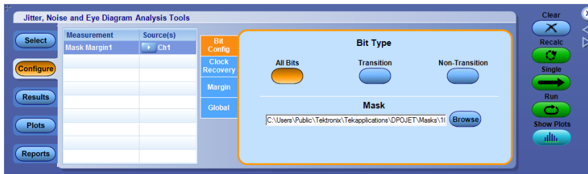
Figure 48: Bit config for mask margin measurement
