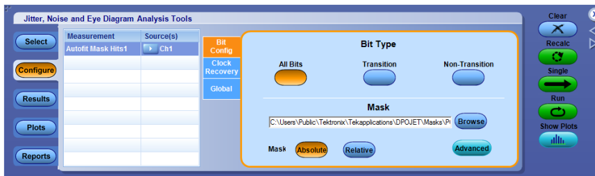
Figure 46: Bit config for autofit mask hits measurement
