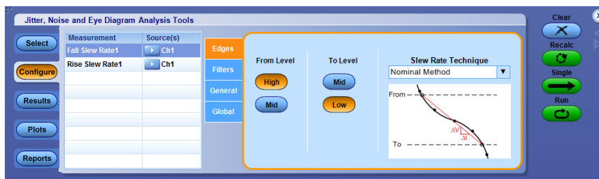
Figure 74: Configuration options for fall slew rate
