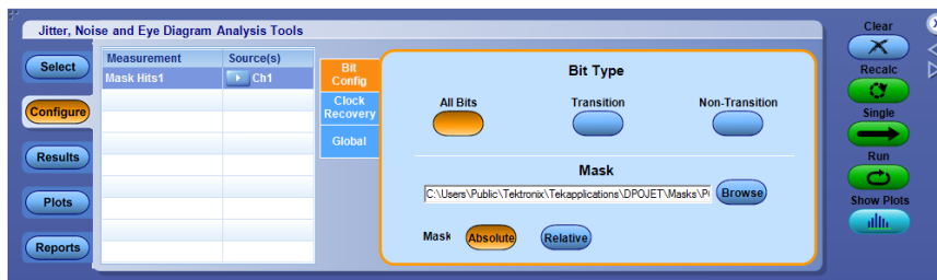
Figure 45: Bit config for mask hits
