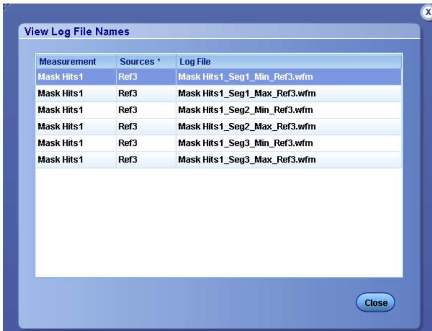
Figure 141: Logging worst case for mask hits measurement
