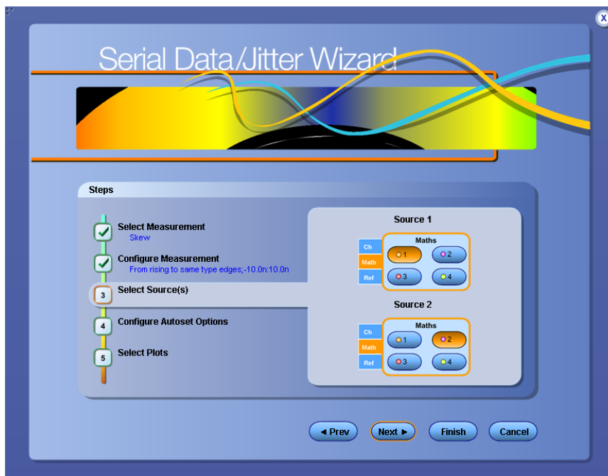
Figure 95: Select sources (Two source measurements)
