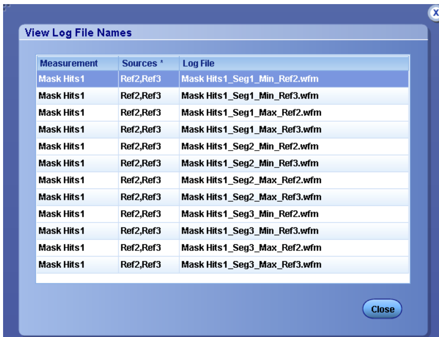
Figure 142: Logging worst case for mask hits measurement (maximum and minimum values)
