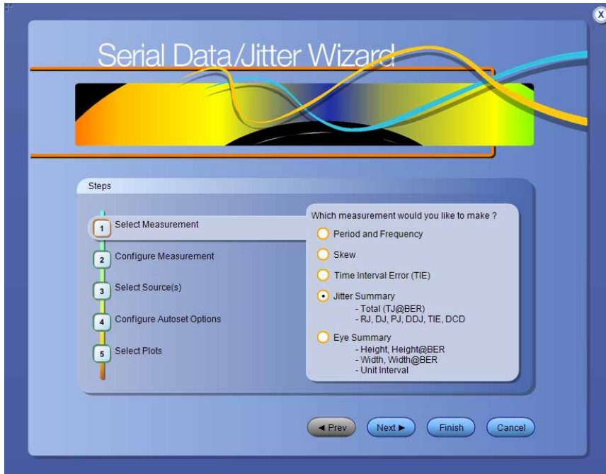
Figure 96: Configure measurement-Jitter summary
