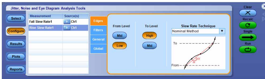
Figure 73: Configuring edges for rise slew rate
