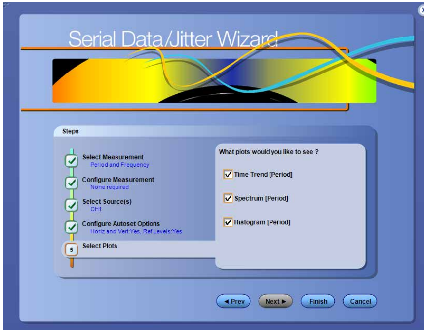
Figure 100: Period and Frequency measurement
