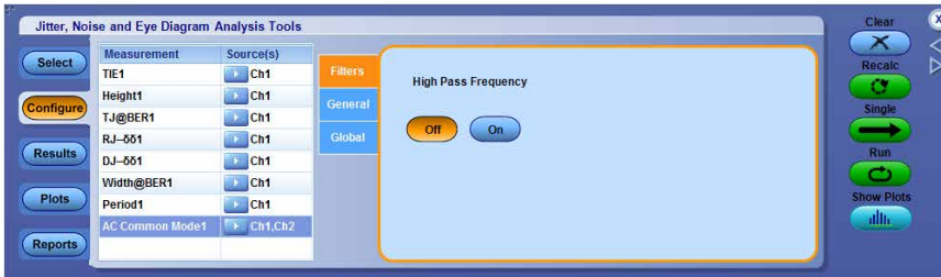
Figure 24: Filter (High Pass Frequency)
