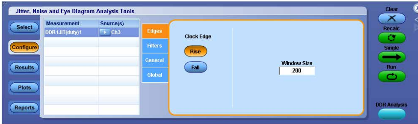
Figure 82: Configuring edges for DDRtJIT(per) DDRtCK(avg) and DDRtJIT(duty)
