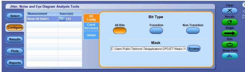
Figure 47: Bit config for mask hits ratio measurement
