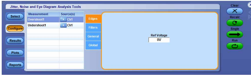
Figure 72: Configuring edges for Overshoot/Undershoot measurements
