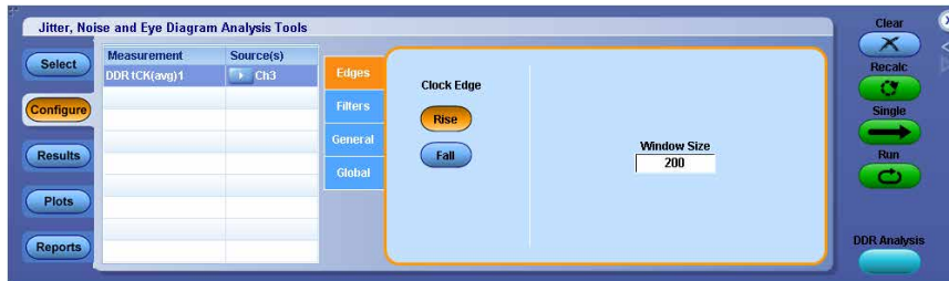
Figure 78: Configuring edges for DDR tCH(avg) and DDR tCL(avg)
