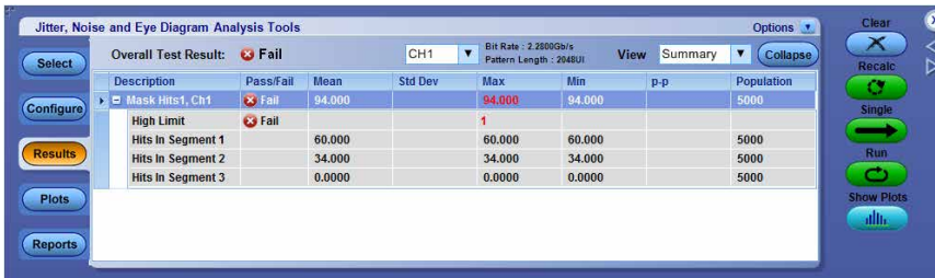
Figure 149: Limits for mask hits (Result)
