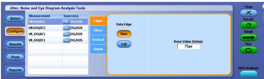
Figure 83: Configuring edges for DDR VIH.DQ(AC), VIH.DQ(DC), VIL.DQ(AC), and VIL.DQ(DC)
