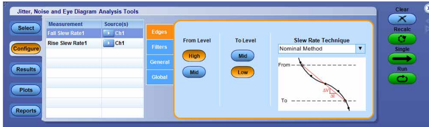
Figure 74: Configuration options for fall slew rate
