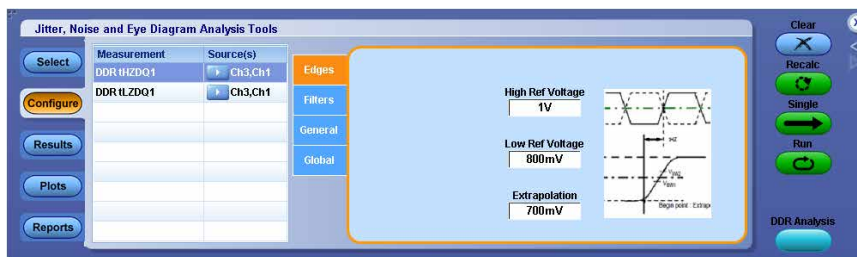
Figure 81: Configuring edges for DDR tHZDQ and DDR tLZDQ
