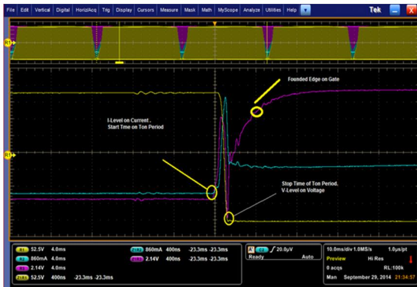
Figure 37: Spike on  $V_g$  source
