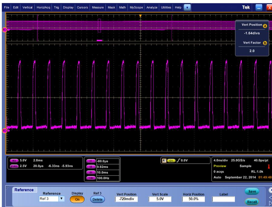
Figure 41: Zoom-in of the (VG) Gate Voltage
