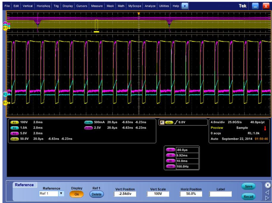
Figure 42: VDS, IDS and VG overlapped
