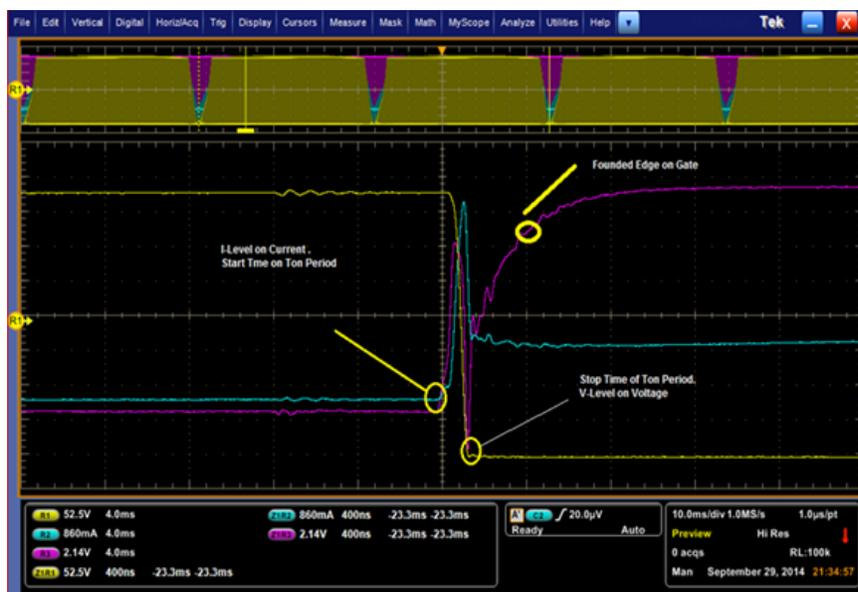
Figure 37: Spike on  $V_g$  source
