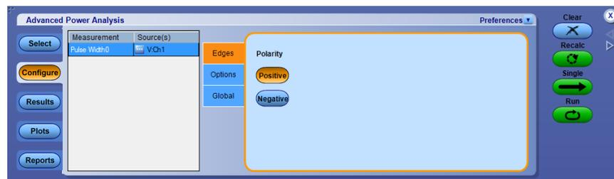
**Control panel** The Control Panel appears on the right of the application window. Using this panel, you can start or stop the sequence of processes for the application and the oscilloscope to acquire information from the waveform.
