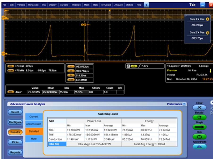
To calculate loss in watts multiply scope built-in value by switching frequency that is 164 KHz, which gives 12.35mW, which lies in within TON loss statistics.
