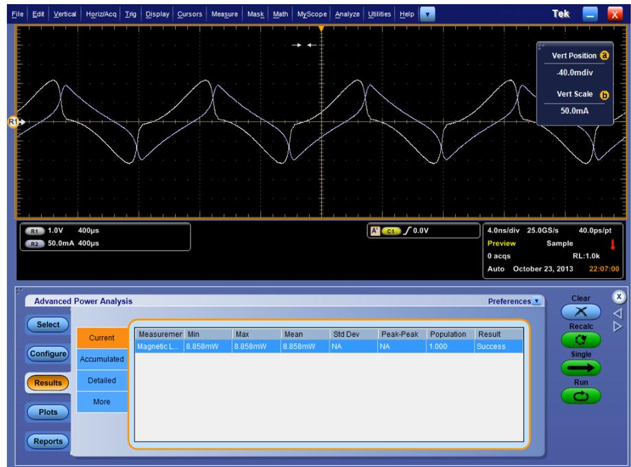
7. The result displays the power loss of the magnetic material.
