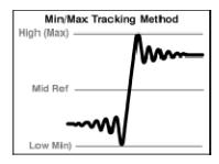
MEAN is commonly used for eye diagrams. The mean method calculates the high value as the mean value of the region above the mid reference and the low value as the mean value of the region below the mid reference. See figure below. The mean is computed only over the eye aperture - typically the center 20% of the NRZ eye, or the center 5% of an RZ eye.
