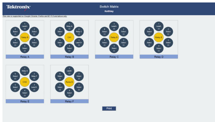
Figure 4: Graphical view of relay cascade configuration
