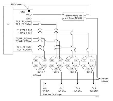
Setup using RF Switch and Tektronix DP-AUX Controller
