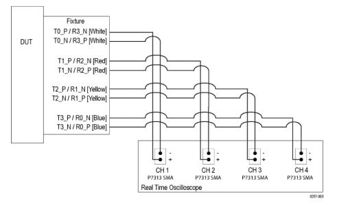
Setup using an RF Switch without Tektronix DP-AUX
