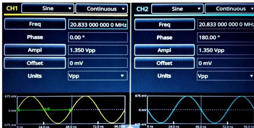
Figure 28: AFG with Test Mode 4 waveform loaded
