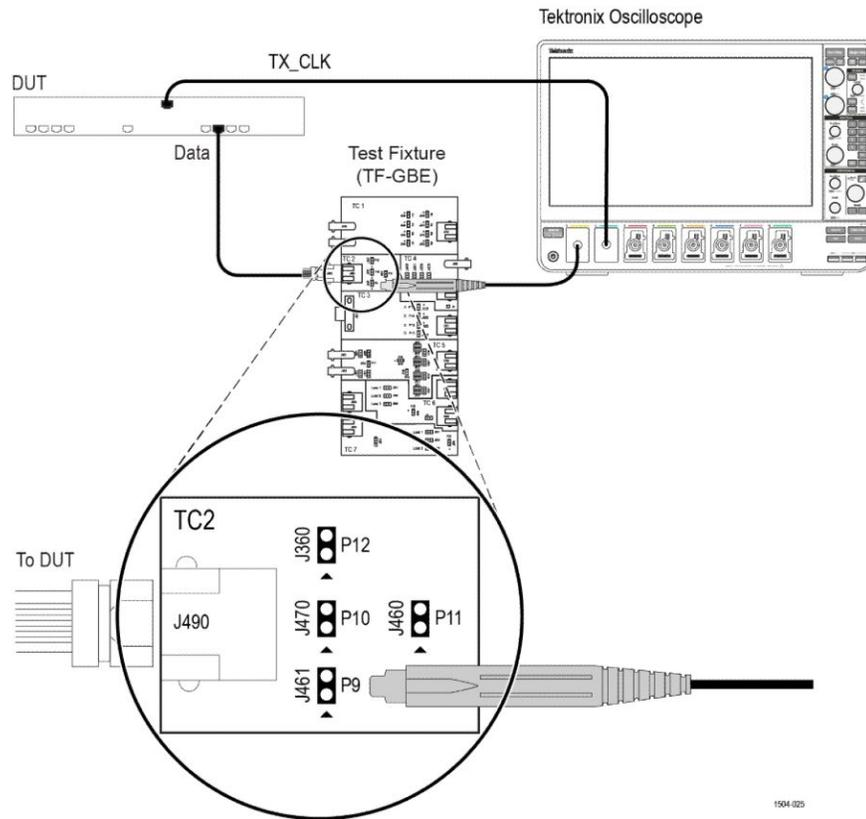
Figure 36: Master Filtered with Clock - Connection 1
