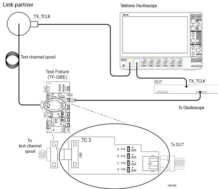
Figure 40: Slave Filtered with Clock - Connection 2
