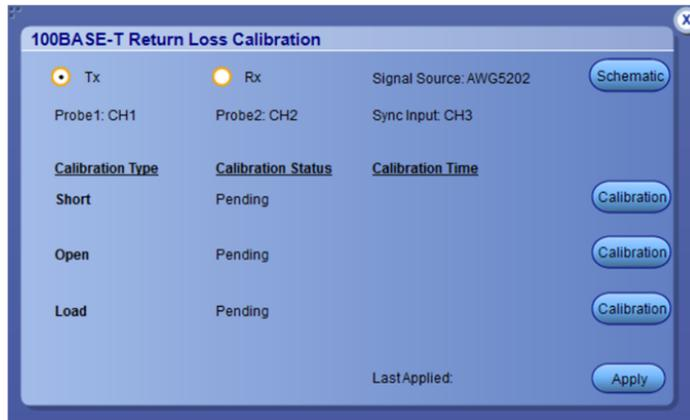
Figure 6: Calibration panel before performing calibration
