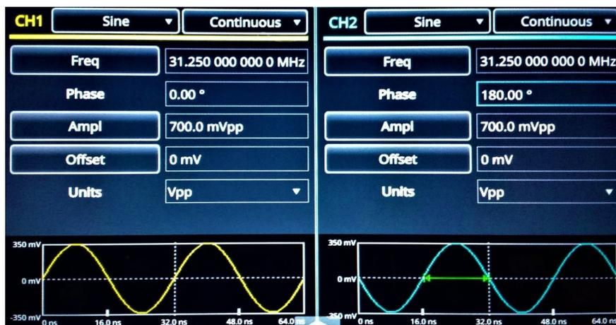
Figure 27: AFG with Test Mode 1 waveform loaded
