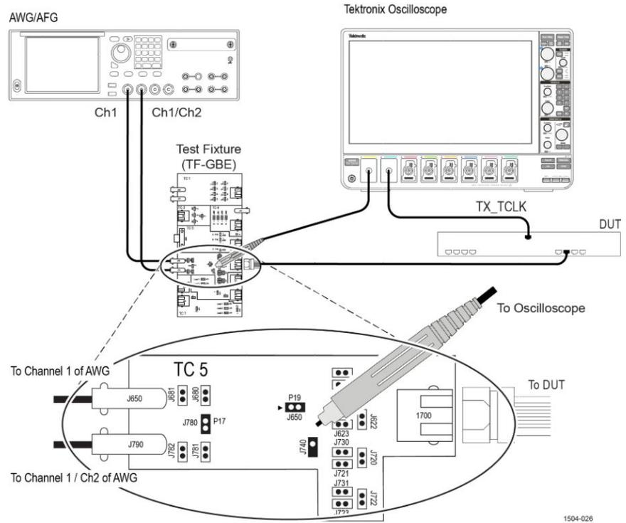
Figure 37: Master Filtered with Clock - Connection 2
