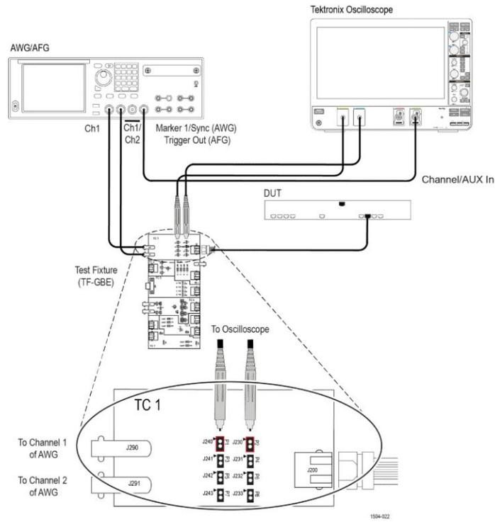
Figure 50: 10BASE-T Transmitter Return Loss
