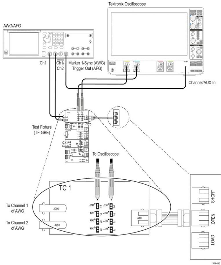
**Figure 10: Connection diagram for OPEN Calibration**
