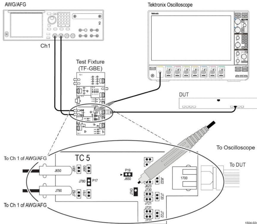
**Figure 22: Connection diagram to measure linearities of the Test Fixture using JigMatch**
