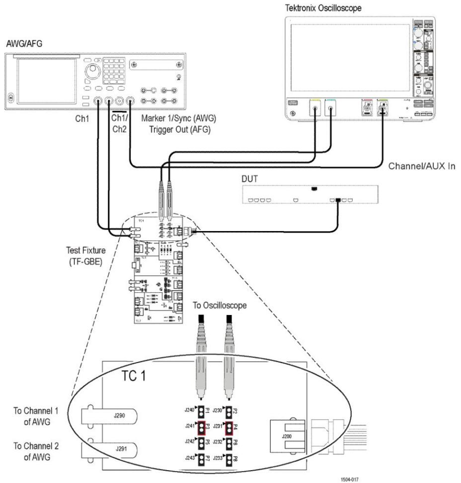
Figure 44: 100BASE-T Receiver Return Loss
