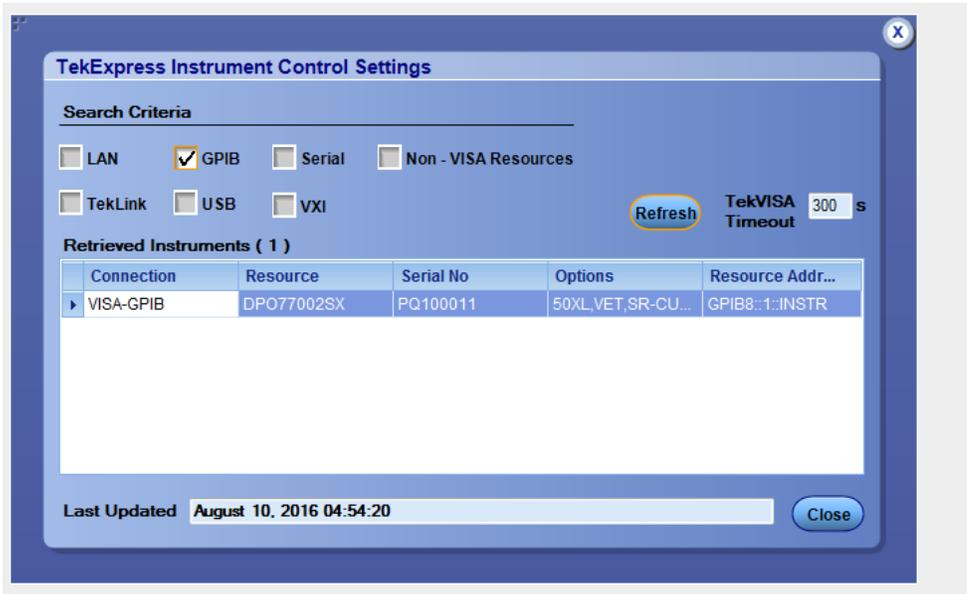
The details of the instruments are displayed in the Retrieved Instruments table. The time and date of instrument refresh is displayed in the Last Updated field.
