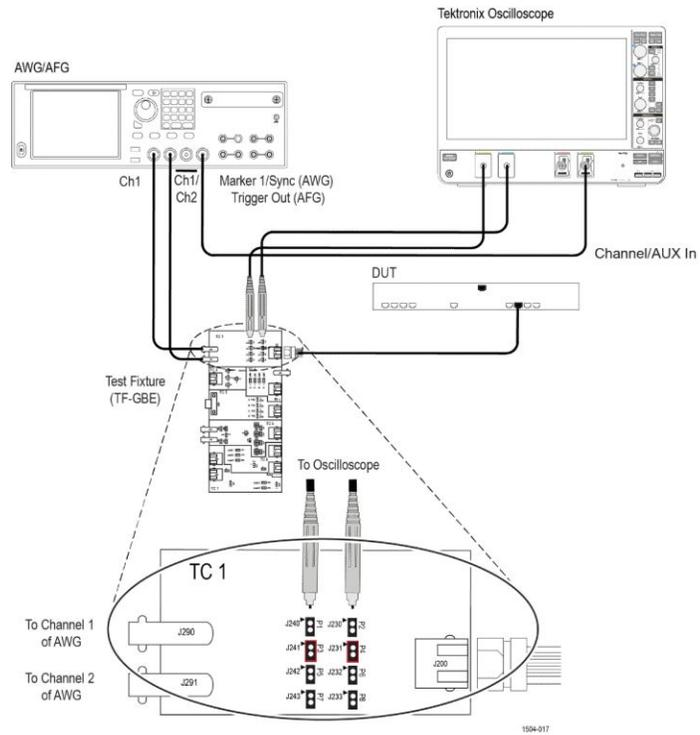
Figure 47: 100BASE-T Receiver Return Loss
