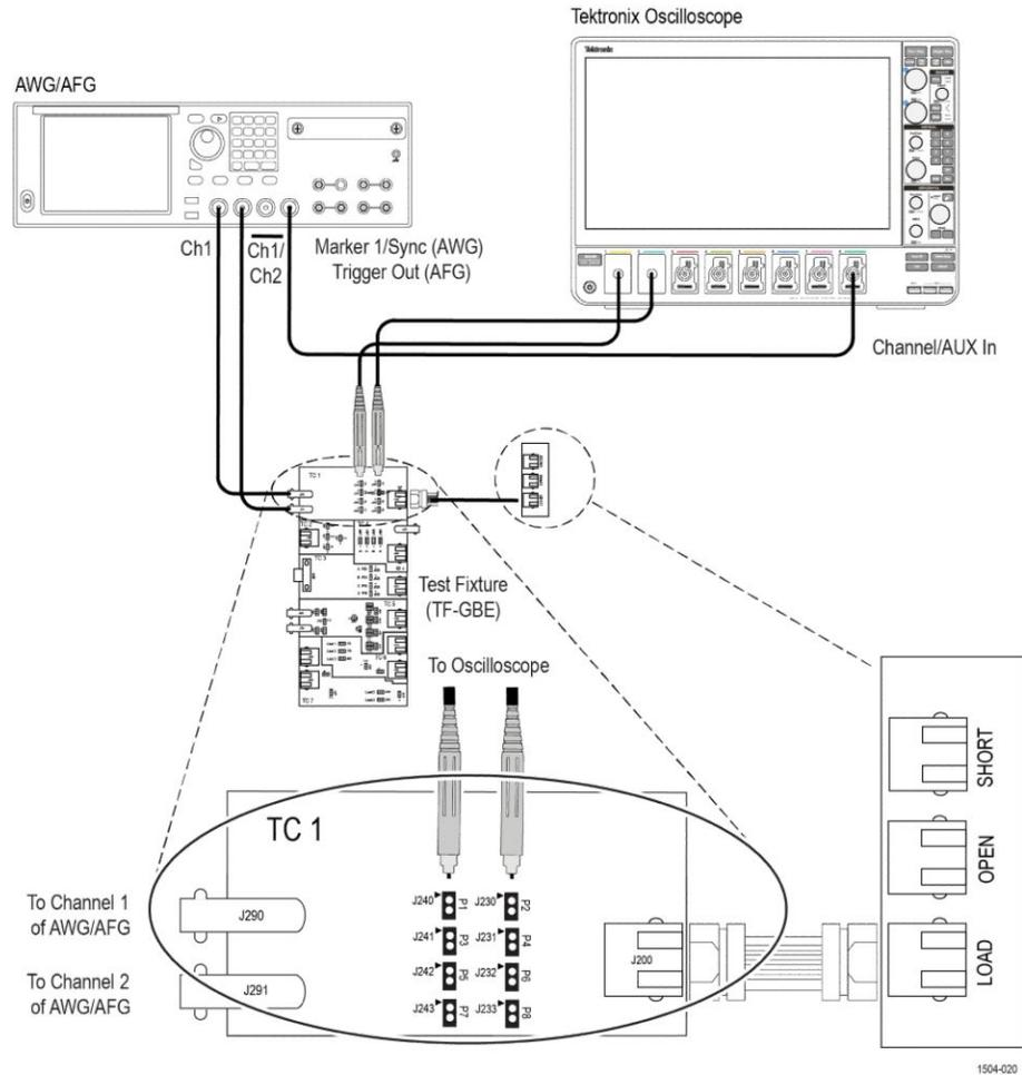
**Figure 12: Calibration output for LOAD calibration**
