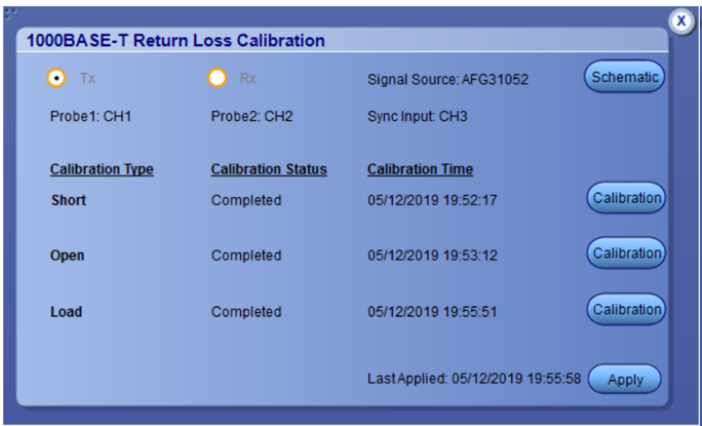
Figure 7: Calibration panel after calibration is performed for OPEN, SHORT, and LOAD and then Apply
