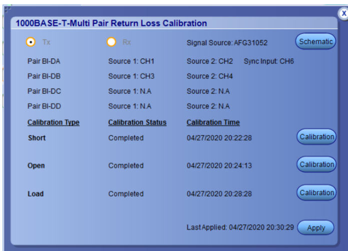
Figure 10: Calibration Panel after calibration is performed for OPEN, SHORT and LOAD, and then Apply for 2 pairs in 1000Base-T-Multi Pair.
