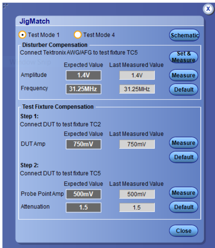
Figure 20: JigMatch calibration configuration panel
