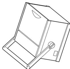
2. Pull the dark grey handle above the logo and lift the keyboard from the device.
