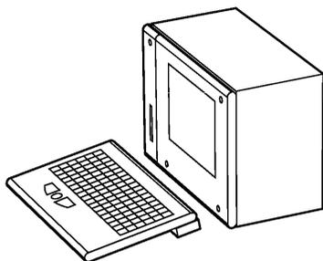
4. Pull on the lower monitor frame to position the monitor in a working angle.
