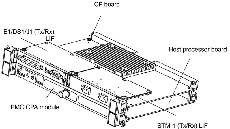
**Figure A-9: ATM PCE I board combination**
