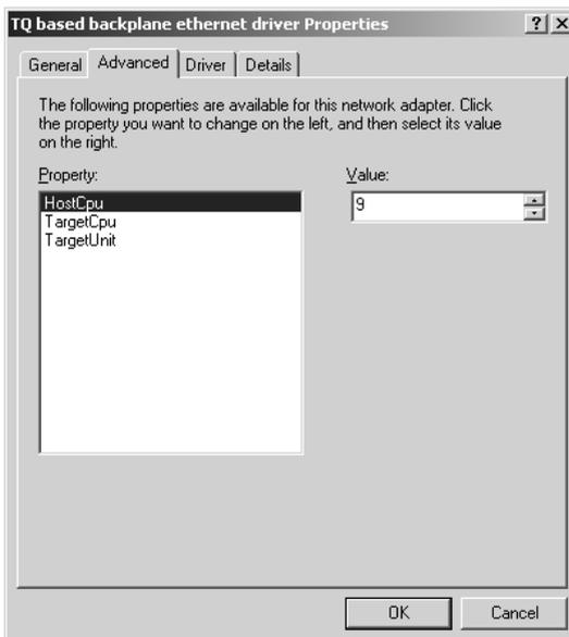
Figure D–9: Configuring the SmEth adapter
