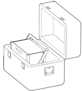
Before closing the transport case make sure that the handle is pointed toward the rear edge of the device.
