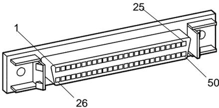
Up to six peripheral devices can be connected to the controller of the system processor via the SCSI socket. Each peripheral device must be assigned an individual address (SCSI ID). The controller occupies address 7 as standard. Since the controller boots from the device with the lowest address, the internal hard disk of the K1297 is set to address 1. When not connected with a peripheral device the SCSI socket is terminated automatically.
