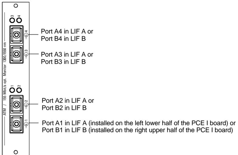
Figure A-12: Front panel of the STM-1 (Rx/Rx) optical line interface
