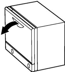
2. Remove the gray cable box from the monitor frame by pulling it away from the device until you hear a loud click: Place both hands at the sides of the cable box and pull the cable box away from the monitor frame. Or place one hand between cable box and monitor frame and press the cable box away from the monitor frame.
