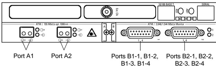
Figure F-6: One STM-1 (Tx/Rx) LIF and one E1/DS1/J1 (Rx/Rx) LIF.
