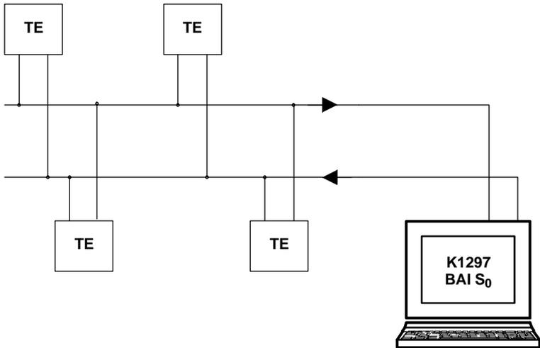
Handsets can be connected so that voice data can be processed bi-directionally in one B channel.
