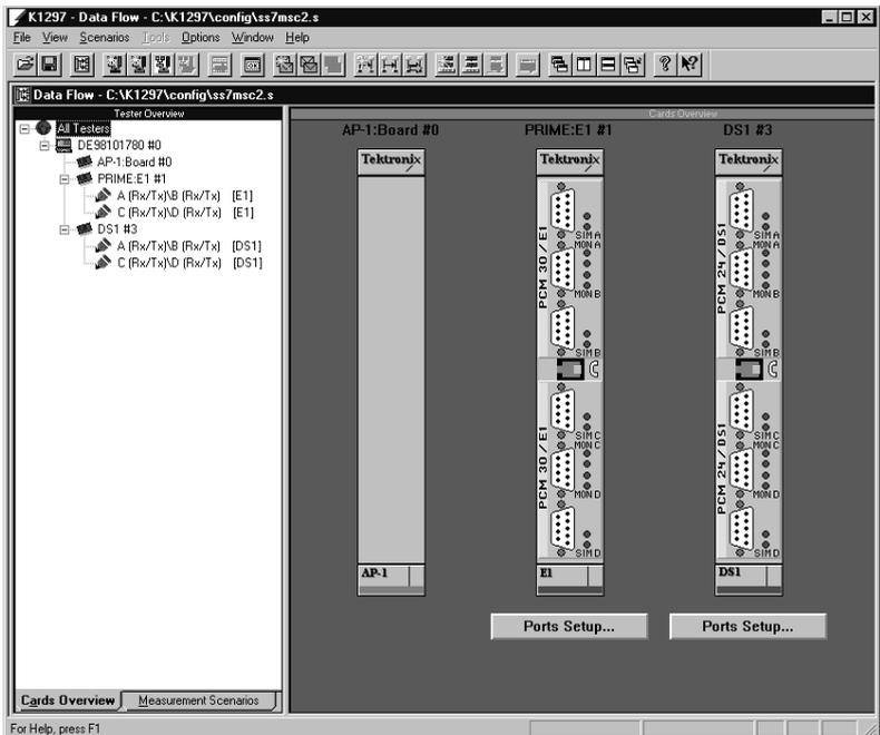
The left pane, *Tester Overview*, displays the interface modules, ports and the line configurations currently set. The right pane, *Cards Overview*, shows the individual sockets on the cards including module designation.
