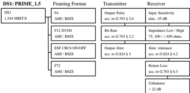
The interfaces of the E1 and DS1 modules implement the physical and electrical connections to the PCM section. For simulation, the sockets feature a transmitter and receiver each for PCM signals. For monitoring, two receivers of the adjacent simulations each are used and combined on a socket.
