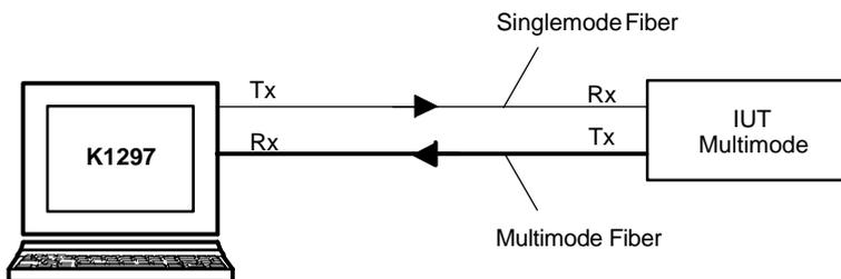
**Simulation / Emulation with Multimode IUTs with Attenuator.** In some cases the optical transmitter of the K1297-G20 overloads the IUT's optical receiver. Typically, in these cases errors on the physical layer (such as bit errors, loss of frame) occur. Inserting an optical attenuator into the connection adjusts the optical power to the sensitivity range of the IUT's receiver.
