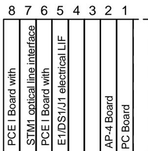
**Figure F-1: Board combination (example)**
