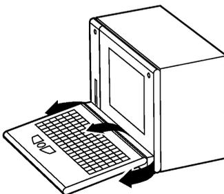
3. Take the cable out of the cable box and fold the cable box underneath the keyboard. The keyboard is now positioned in a working angle in front of you.
