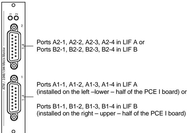
Figure A-14: Front panel of the E1/DS1/J1 (Rx/Rx) electrical line interface
