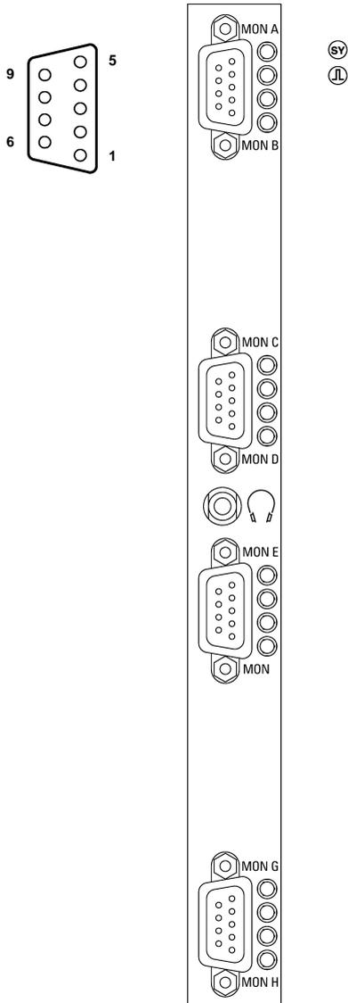
Figure A-6: E1/DS1 monitoring board (PRIMO)
