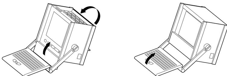
2. Press the lateral handle hinges (variant handle: push up hinges) and put the handle into a vertical position.
