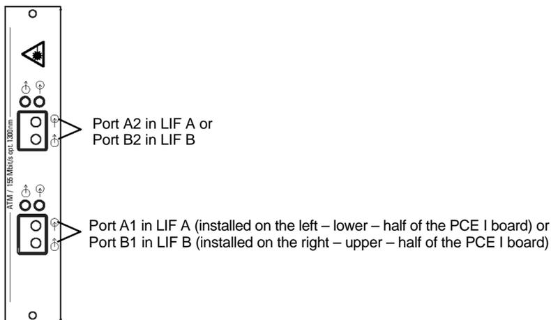
Figure A-11: Front panel of the STM-1 (Tx/Rx) optical line interface
