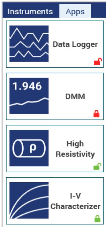
When you first open KickStart, the Instruments tab displays available instruments on the left. Select the Apps tab and you will see a lock on each App. The text below describes the licenses and lock icons:
