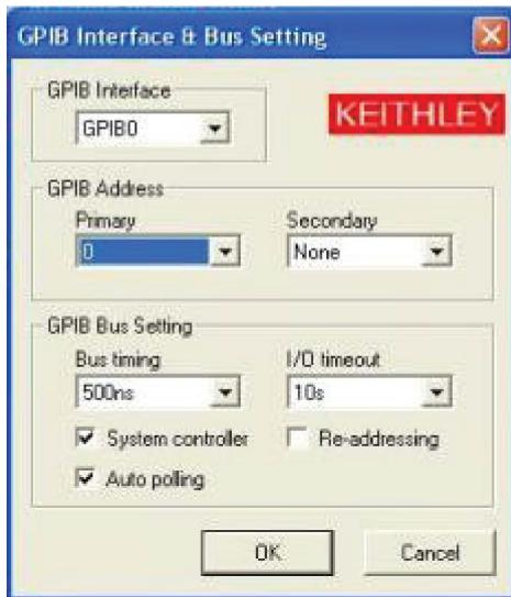
5. Save these configuration changes by selecting **Setting > Save Configuration** in the Keithley GPIB Configuration Utility window.
