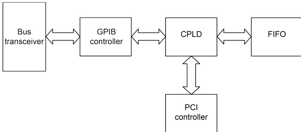
The FIFO can buffer data from the master (either from the KPCI-488LPA or external device) when the target is busy. Therefore, the efficiency will be significantly improved when transferring large blocks of data.
