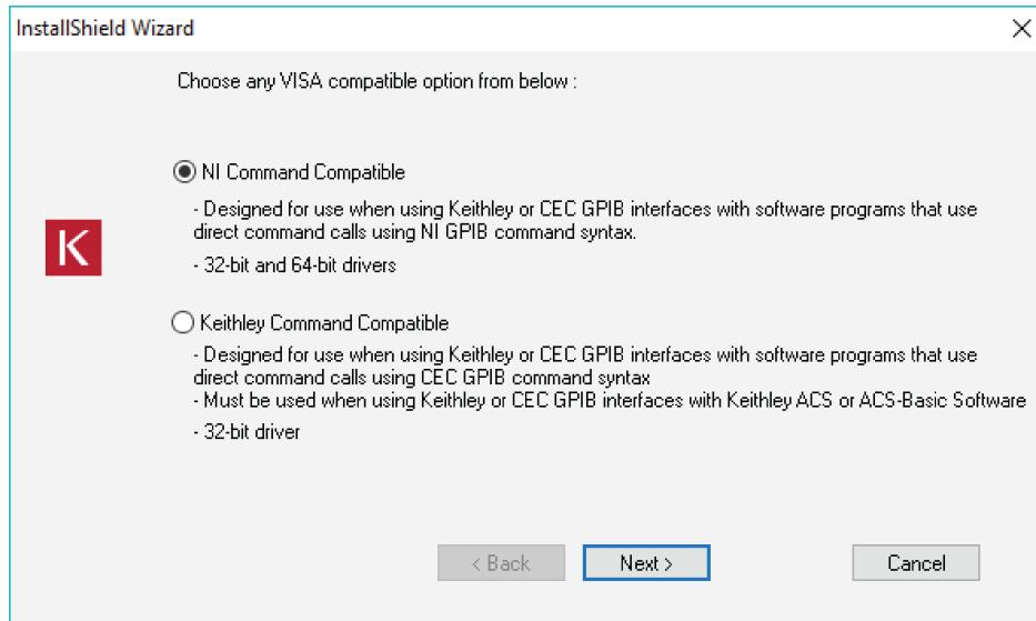
6. Install one of the following drivers. The InstallShield Wizard provides guidance on which driver to install.
