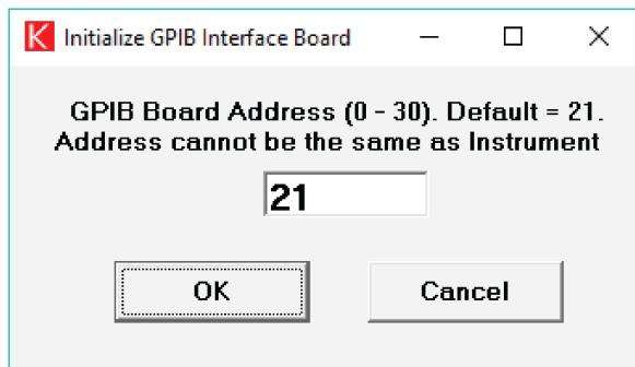
2. Enter the address to assign to your GPIB interface. The default is 21.
