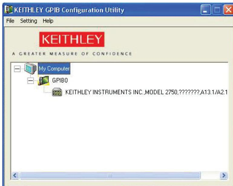
3. Double-click the interface icon to open the GPIB Interface & Bus Setting dialog box.
