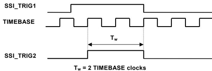
As an input, the Model KPXI-AI-2-65M accepts the SSI\_TRIG2 signal to be the source of a one-clock delayed trigger event. The controller on the Model KPXI-AI-2-65M will then compensate the one-clock delay if using SSI\_TRIG2 as the source of trigger event. The signal is configured in the rising edge-detection mode.
