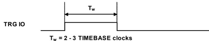
When the Model KPXI-AI-2-65M is plugged into the star trigger controller slot, i.e. slot 2, in a PXI system, it can export trigger signals to other 13 generic peripheral slots (PXI\_STAR0 ~ PXI\_STAR12) through the PXI star trigger pin. The trigger signal source can be from software trigger, external digital trigger signal from TRG IO, analog trigger and PXI Trigger Bus[0:7]. The output trigger signal timing characteristic is identical to the TRG IO which is shown in [Figure 3-21](#).
