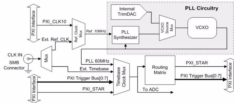
Once you have chosen the timebase source, you can set a 24-bit counter to divide the timebase to get the needed sampling rate. The following formula determines the ADC sampling frequency:
