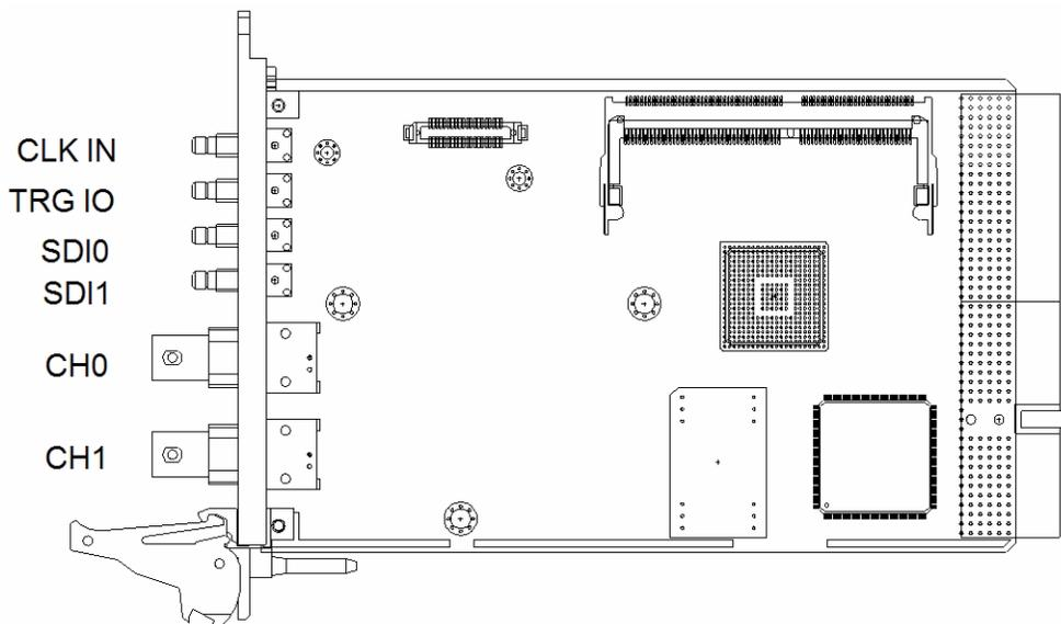
The Keithley Instruments Model KPXI-AI-2-65M module is packaged in a Eurocard form factor compliant with PXI Specifications measuring 160mm in length and 100mm in height (not including connectors). The connector types and functions are described as follows.
