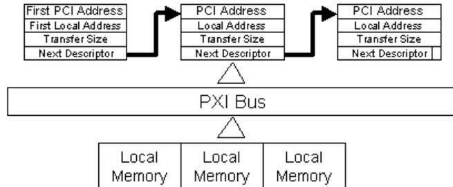
If the data throughput from the Model KPXI-AI-2-65M is less than the available PCI bandwidth (For example: 20MS/s \* 2 channels \* 2 Bytes/channel = 80MB/s), the Model KPXI-AI-2-65M also features on-board 3k-sample FIFO to achieve real-time transfer bypassing the SDRAM, directly to host memory.
