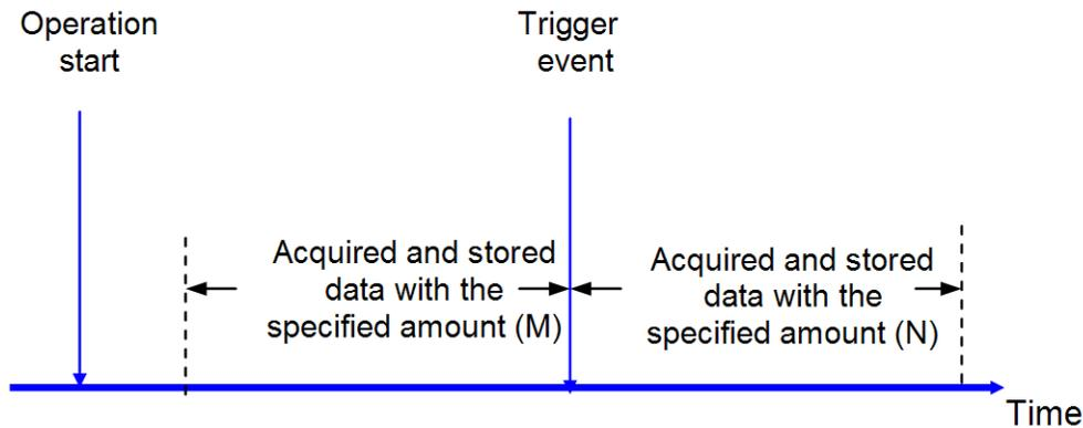
Like pre-trigger mode, the stored data may be less than the amount specified if the trigger event occurs before the specified amount of data (M) has been acquired. Users can also set by program to ignore trigger signals until the specified amount of data (M) has been acquired.
