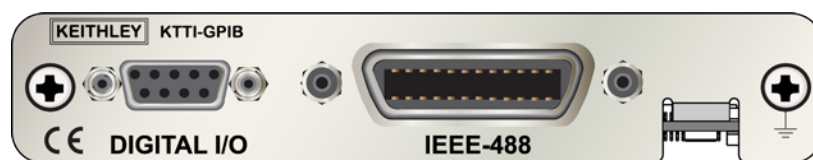
Figure 2: KTTI-GPIB connector view
