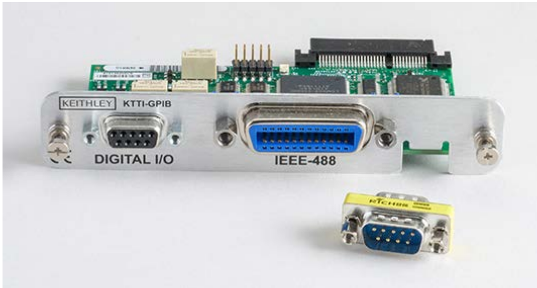
Figure 1: KTTI-GPIB communications card
