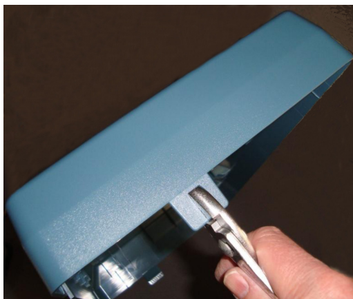
Figure 2: Removing tabs from the front protective cover
