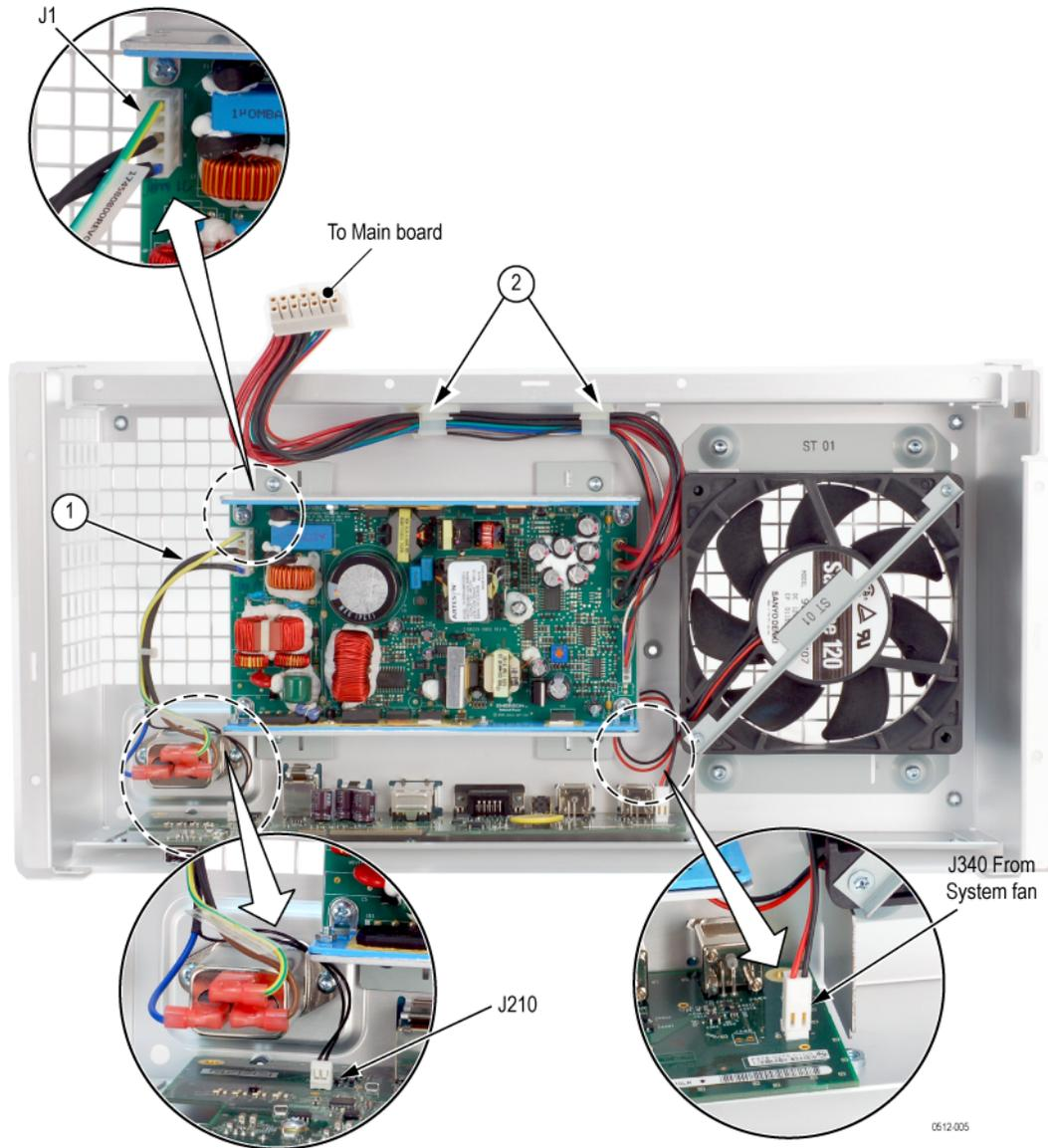
Figure 11: Rear chassis, showing cables and connectors
