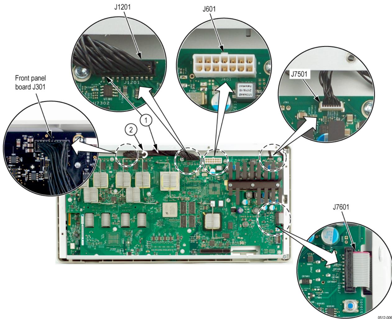
Figure 12: Main board, showing cable and connectors
