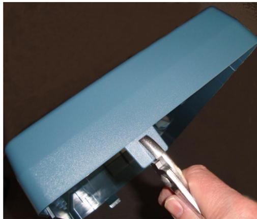
**Figure 2: Removing tabs from the front protective cover**
