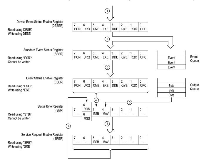
When an event occurs, a signal is sent to the DESER (1). If that type of event is enabled in the DESER (that is, if the bit for that event type is set to 1), the appropriate bit in the SESR is set to one, and the event is recorded in the Event Queue (2). If the corresponding bit in the ESER is also enabled (3), then the ESB bit in the SBR is set to one (4).
