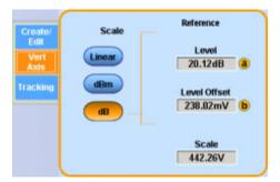
**NOTE.** The reference level offset is used to calculate the log magnitude in dB. Adjusting the reference level positions the waveform with respect to the top of the screen but does not change the position of the waveform with respect to the ground reference marker.
