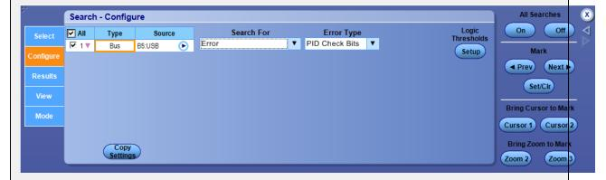
Select the Error Type from the drop-down list. Click Setup to adjust the logic thresholds.
