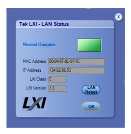
**NOTE.** Pushing the LAN Reset button does a LAN configuration initialization: enables DHCP, enables Auto-IP, enables ICMP ping responder, sets the Web password to default (No password), and updates the LXI XML identification. Refer to the LXI specification for more information.
