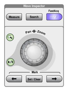
Use Measure to perform automated measurements, Search to search through an acquisition for user-defined events/criteria, or DPX/FastAcq to start or stop fast acquisitions.
