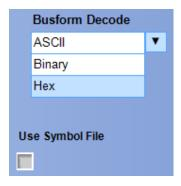
For the USB serial bus, you can display the decode of the bus in Mixed Hex, Mixed ASCII, Hex, Binary, Packet, and Details. The speed you select determines the available decodes. Select the decode form the drop down list.
