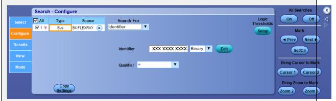
Select the Identifier from the drop-down list. Click Edit to enter the value. Click Logic Thresholds to adjust the logic thresholds.
