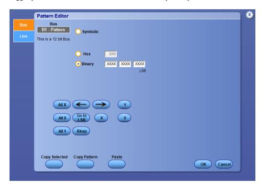
When you select a serial bus and click the Edit button, use the Pattern Editor controls to set up the bus trigger pattern for a serial bus value. For example, the Data (SPI bus), or the Address, Data, or Address and Data (I2C bus) bus values.
