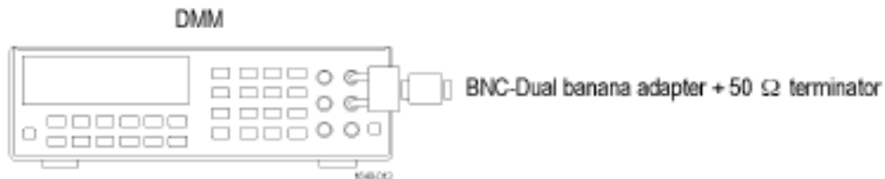
Figure 5: 50 Ω terminator accuracy
