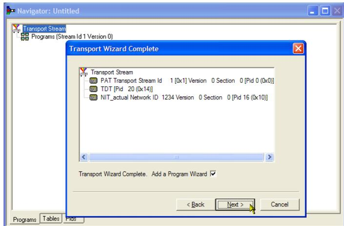
**Elementary stream acquisition.** For this example, you need to add a video and an audio elementary stream to the transport stream that you have created. You can extract suitable streams from one of the sample transport streams supplied with the MTS4000 installation. The stream used in this example is Sym1.mpg. This file is available on the hard drive of the MTS4000, the Tclips MPEG Test Streams DVD, and the Documentation CD.
