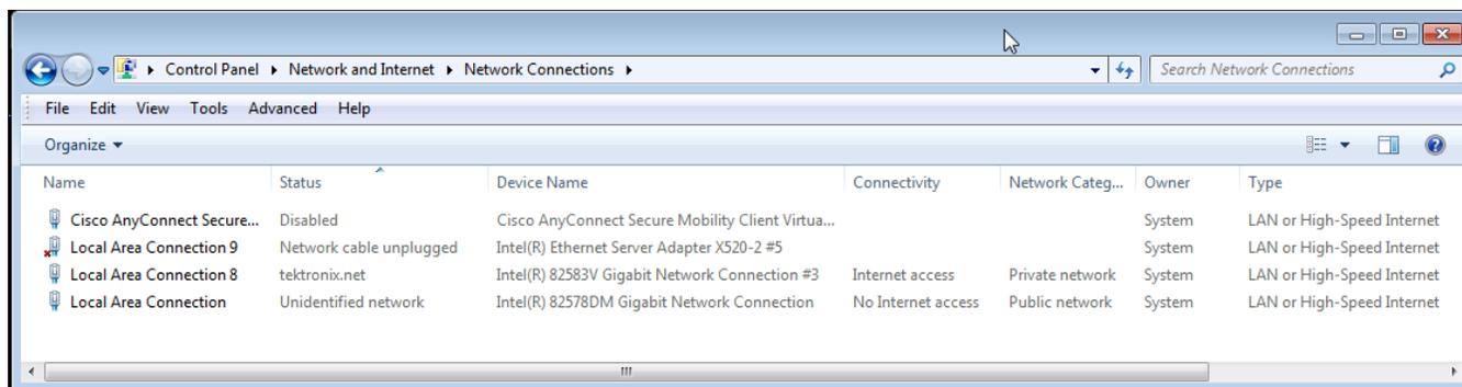
**Upper NIC.** The upper NIC has a device name of Intel 82583V and is normally used for LAN and MS RDP remote control. The I/O bandwidth limitations of this NIC are:
