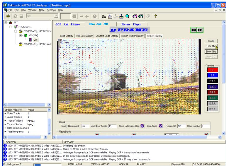
Additionally, you can see the characteristics of any of the macroblocks that make up the picture by hovering the mouse over a picture macroblock.
