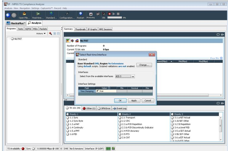
2. In the Select Real-time Interface dialog screen, select an available input from the Interfaces pull-down menu.
