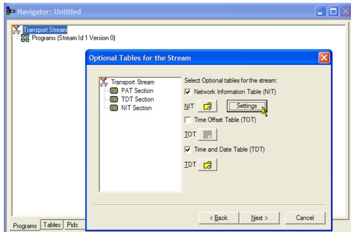
17. In the Set up the NIT dialog box, enter the Network Id 1234 and the Network Name Tek\_test.
