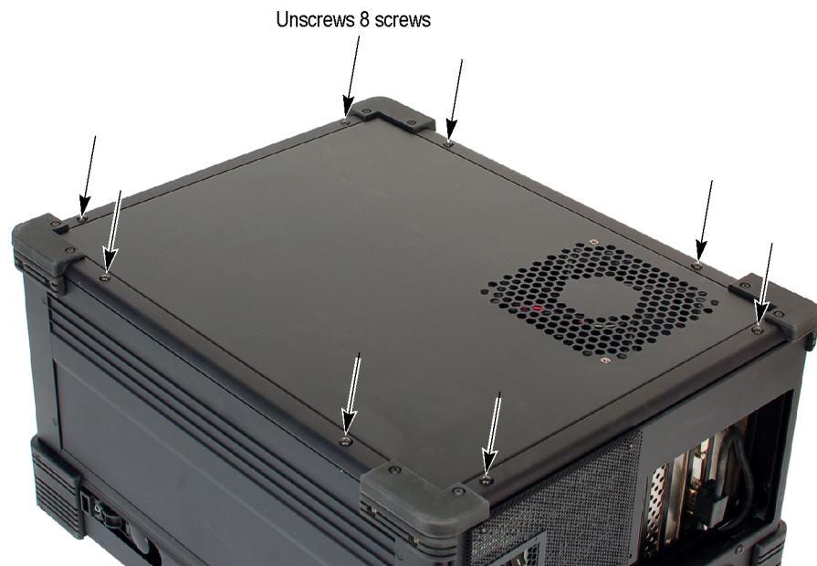
Figure 3: Remove rear panel
