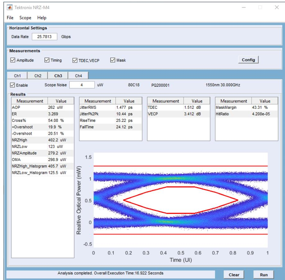
This application is intended to be installed on a PC and works by connecting to the sampling scope. Application allows you to acquire signal directly from the connected DSA8300 sampling oscilloscope and analyze the acquired waveform data.
