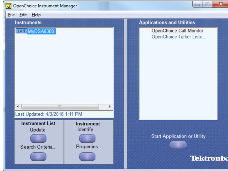
To detect an instrument for through TekVISA, select the Search Criteria button and then select LAN. Search on the IP address.
