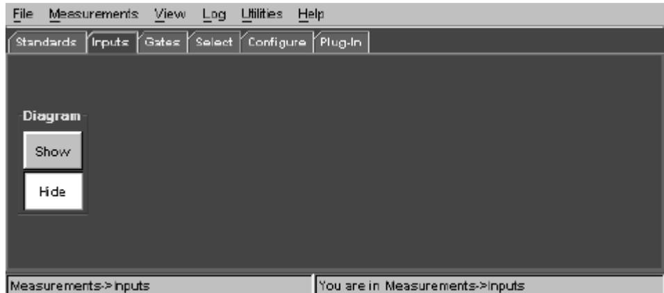
To display input parameter fields, select the Diagram Show button to display the Inputs Block Diagram (IBD) and then select a button. The Measurements Input menu then updates to display the parameter fields associated with the selected IBD button. For example, the following figure shows the Data Signal input parameters, which are displayed after selecting Data Signal on the IBD.
