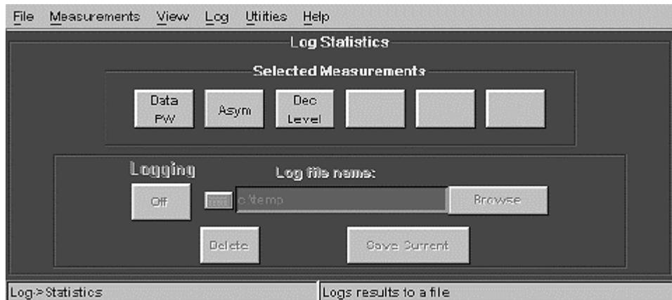
2. Select the measurement button in the Selected Measurements area to select the measurement to log. You can log up to six measurements at a time, but you must select and enable each measurement for logging.
