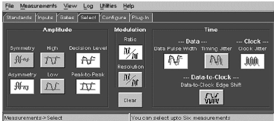
2. Select the measurements you want to take. You can select up to six measurements, in any combination, from any of the measurement type groups.
