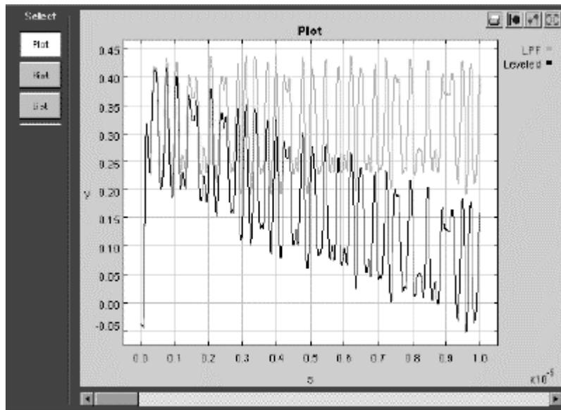
If you are measuring from the LPF output then a good initial value for the Slicer Initial Threshold parameter is the Autoset calculated data Threshold parameter value. Viewing the LPF signal (which is the Slicer input) also gives good basis for estimating an Initial Threshold value for the slicer.
