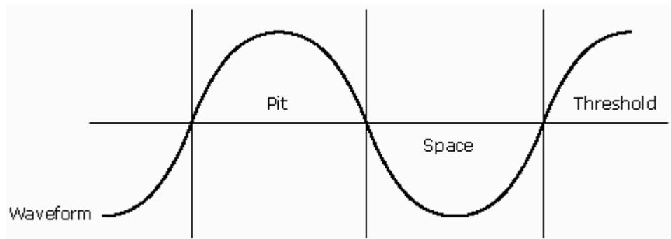
The data signal waveform is first processed to identify the pits and spaces, the parts of the processed read-back waveform corresponding to the physical pits and spaces embossed on the media. Each waveform segment, delimited by threshold crossings, is a data pulse. The waveform segments are categorized as pits or spaces, depending on the polarity of the voltage corresponding to this data pulses (with respect to the threshold level).
