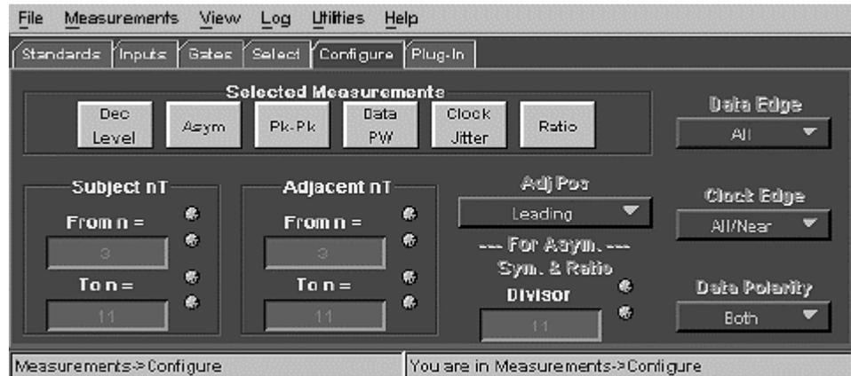
To configure a selected measurement, select the button corresponding to a selected Measurement, and adjust the parameter values. Note that you cannot set different parameter values for each measurement. For example, you cannot set the Adj Pos value to Leading for one measurement and then set it to Trailing for a different measurement. All measurements will use the last values entered in the parameter fields.
