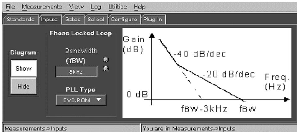
Use the general purpose knob or keyboard to change a value. Refer to Phase-Locked Loop Parameters on page 91 for information on the Bandwidth and PLL Type parameter values and ranges.
