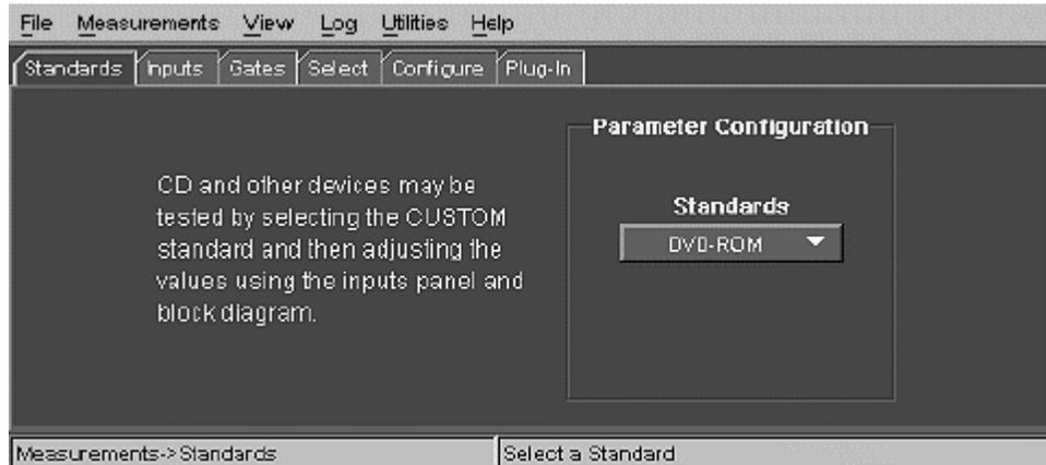
If you are testing for a standard that is not in the list, select Custom from the list. Then use the Inputs, Gates, Select, and Configure menus to set your custom measurement parameters. You can then save the custom measurement settings by selecting File > Save/Recall and specifying a file name and directory in which to store the settings.
