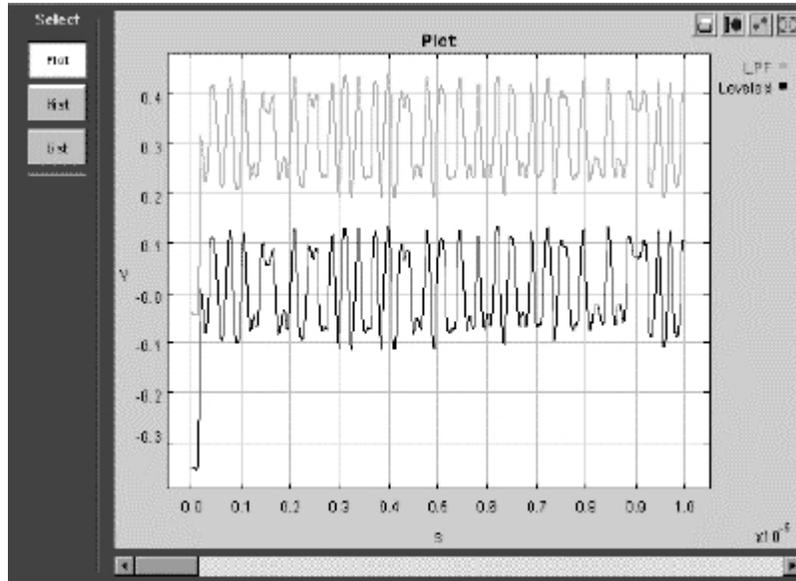
If the Slicer Initial Threshold parameter is incorrect, the Leveled signal is not centered on zero volts, but slowly adjusts to the zero volt level depending on the Slicer bandwidth value, as shown in the below figure.
