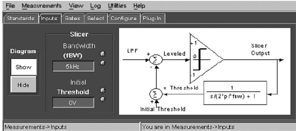
4. Use the general purpose knob or keyboard to change a value. Refer to Slicer Parameters on page 90 for information on the Bandwidth and Initial Threshold parameter values and ranges.
