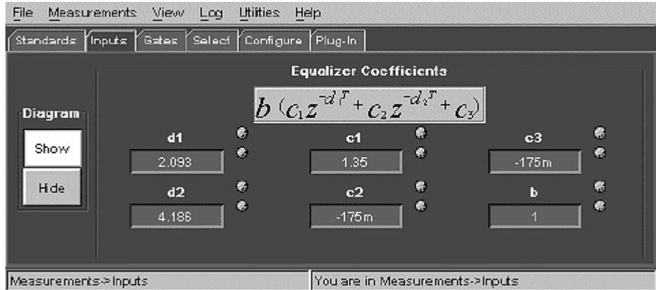
4. Use the general purpose knob or keyboard to change a value. Refer to Equalizer Coefficient Parameters on page 90 for information on the equalizer parameter values and ranges.
