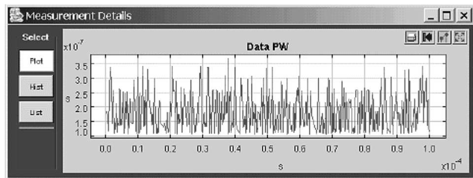
The available measurement display formats are Plot, Hist (histogram), and List. Other functions within this frame let you save measurements to a file, set the histogram bin value, autofit or format the plot X and Y values, and print the measurement information.
