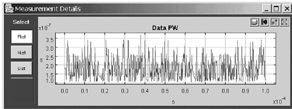
3. In the Measurement Details area, select the Hist button. The area redraws the data as a histogram, as shown below.
