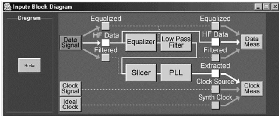
You configure the signal path by selecting the buttons. Selecting a button either changes the signal path route or displays fields in which to enter signal input and processor parameters. To close the IBD, select Hide.
