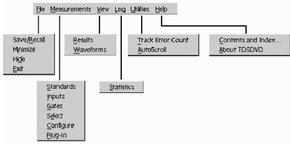
You can also select menu items from the keyboard by pressing and holding the Alt key in combination with the letter underlined in the menu or submenu item. For example, to use the keyboard to display the Measurements > Configure panel, press and hold the Alt key, press the M key, and then press the C key.
