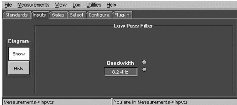
4. Use the general purpose knob or keyboard to change the value. Refer to Low Pass Filter Parameters on page 90 for information on the Bandwidth parameter values and ranges.
