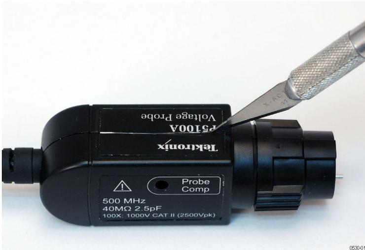
Figure 3: Cut the two side labels in half
