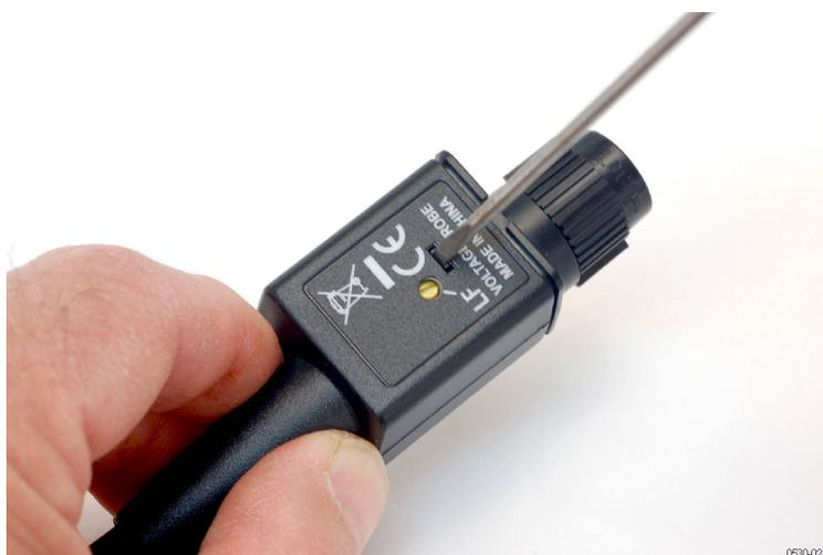
**Figure 13: Depress the tab and slide back the cover**
