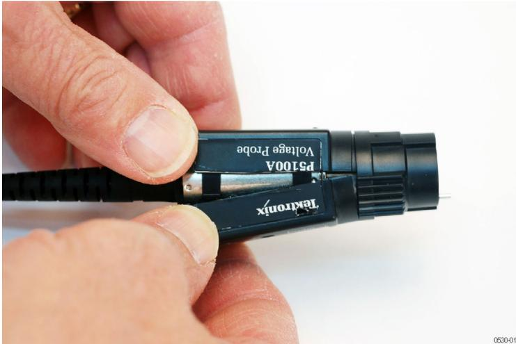
**Figure 5: Remove the top cover from the probe**
