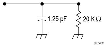
**Figure 11: P5910 probe loading and equivalent circuit**
