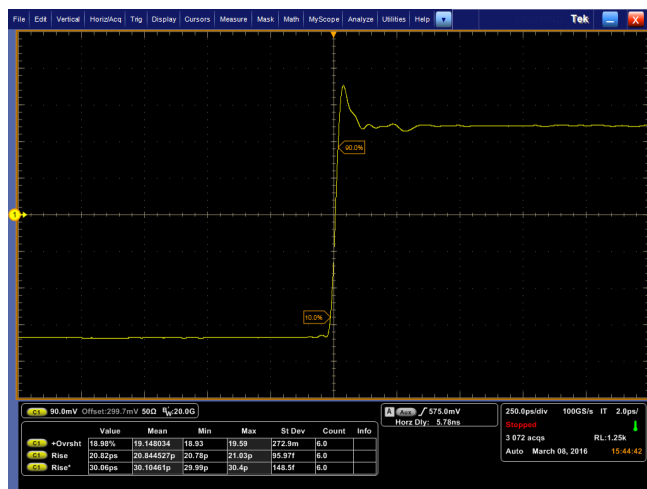
Figure 20: P77STFLXA solder tip attached with 120 mils (3.05 mm) wires (rise time = 30.1 ps)
