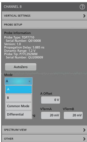
**A-B mode** The A-B Mode is used for making differential signal measurements and represents the traditional differential probe functionality. Since the A-B Mode measures the difference between the A and B input signals, it eliminates any common mode voltage, such as a DC bias common to both inputs, within the CMRR performance capability of the probe.
