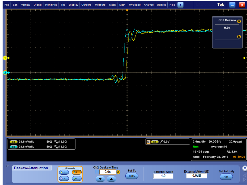
Figure 5: Signal delay between two channels
