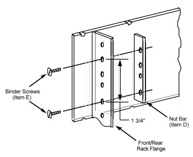
3 Repeat previous step on the rear rack flanges. These nut bars should be mounted at the same level and oriented the same way as those in front.
