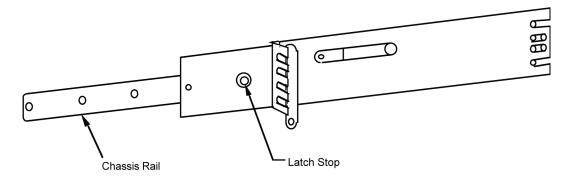
Attach each rail to the instrument chassis with four 10-32 3/8" Phillips flat head screws (item F). When mounting the Model 707 facing forward, use the front four holes on the chassis. See the following figure. The Model 707 can also be mounted with its rear panel at the front of the rack. In this case, use the rear four holes.
