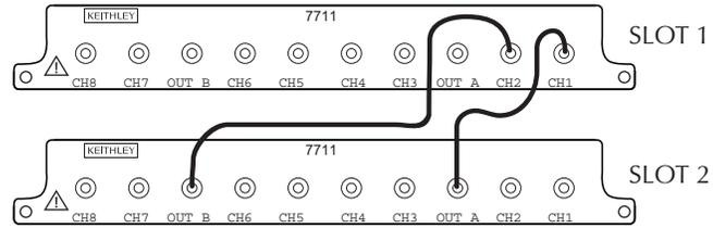
NOTE: The simplified schematic is shown in the power up state (Channels 1 and 5 are closed for cards in slots 1 and 2).
