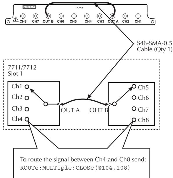
NOTE: The simplified schematic is shown in the power up state (Channels 1 and 5 closed).
