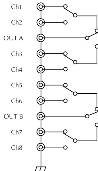
**NOTE** To close channels 1 and 5 on a Model 7711/7712 in slot 1, send: `:ROUT:MULT:CLOS (@101,105)`
