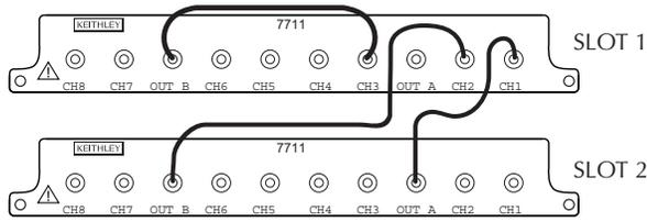
NOTE: The simplified schematic is shown in the power up state (Channels 1 and 5 are closed for cards in slots 1 and 2).
