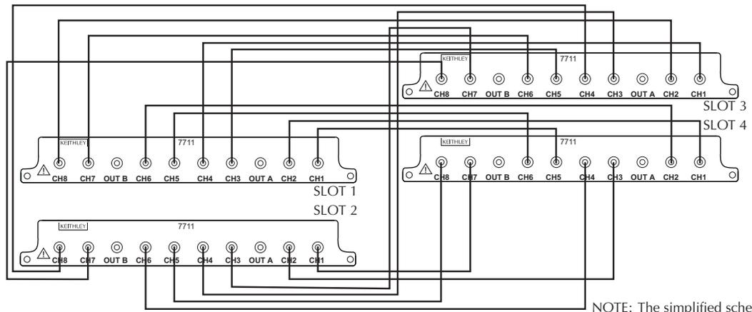
NOTE: The simplified schematic is shown in the power up state (Channels 1 and 5 closed for cards in all slots).
