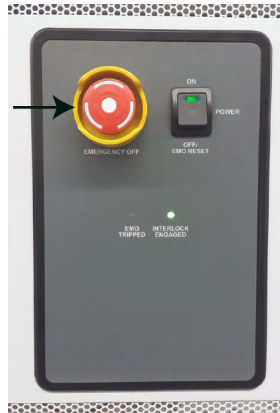
Figure 42: EMERGENCY OFF button
