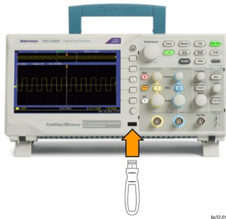
**Figure 28: Import the package from your USB memory device into your TBS1000B-EDU oscilloscope**
