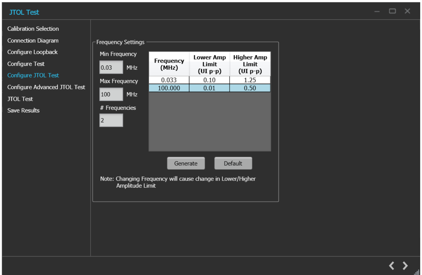
JTOL Test: Configure JTOL Test
