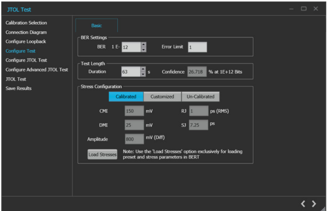
JTOL Test: Configure Test
