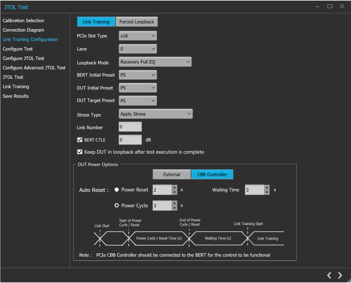
Figure 70: JTOL Test: Link Training Configuration (Link Training-CBB Controller)
