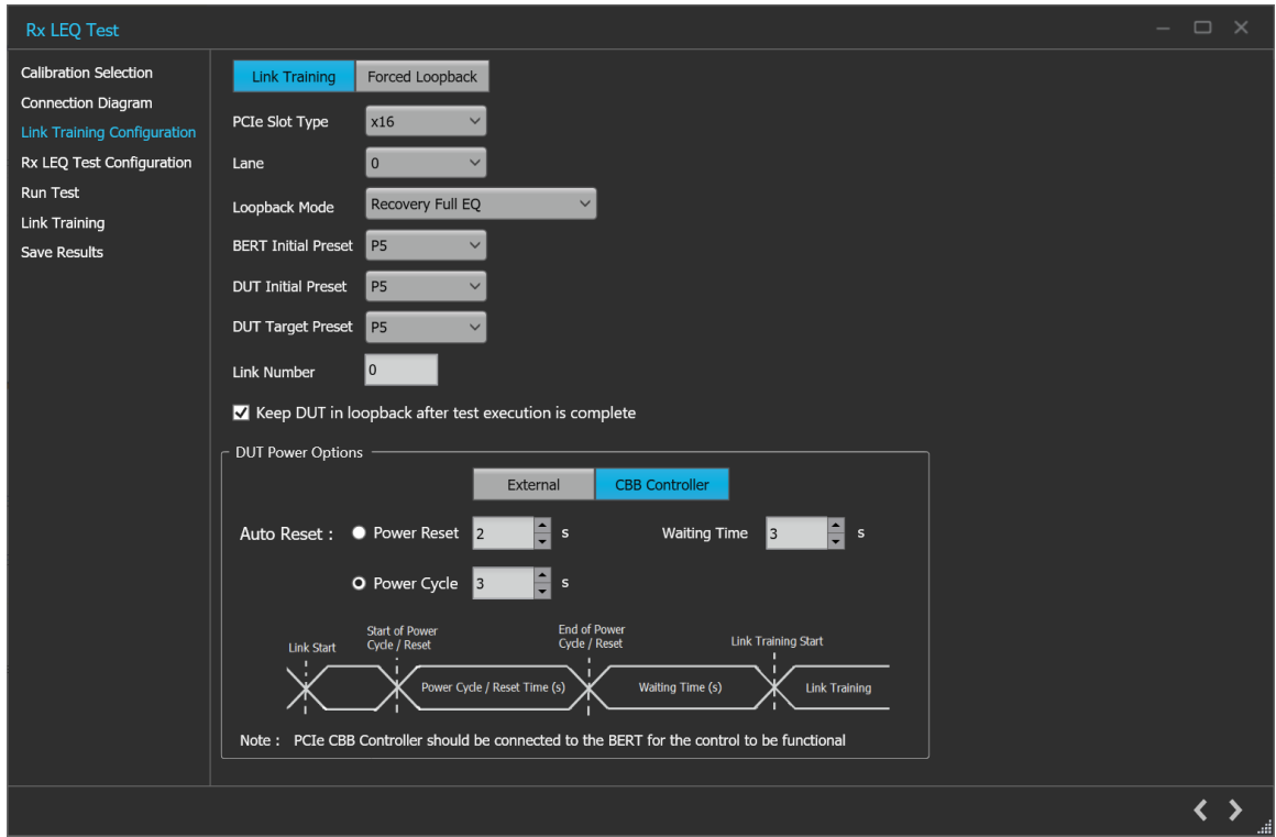
Figure 46: Rx LEQ Test: Link Training Configuration (Link Training-CBB Controller)
