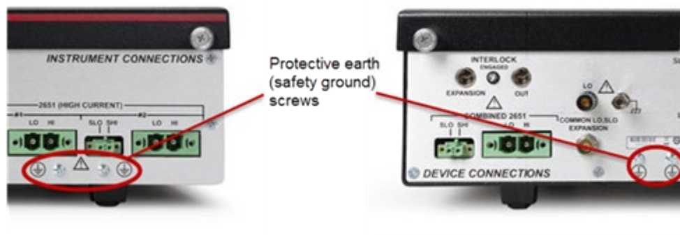
Figure 80: Protective earth (safety ground) screw locations on the Model 8020
