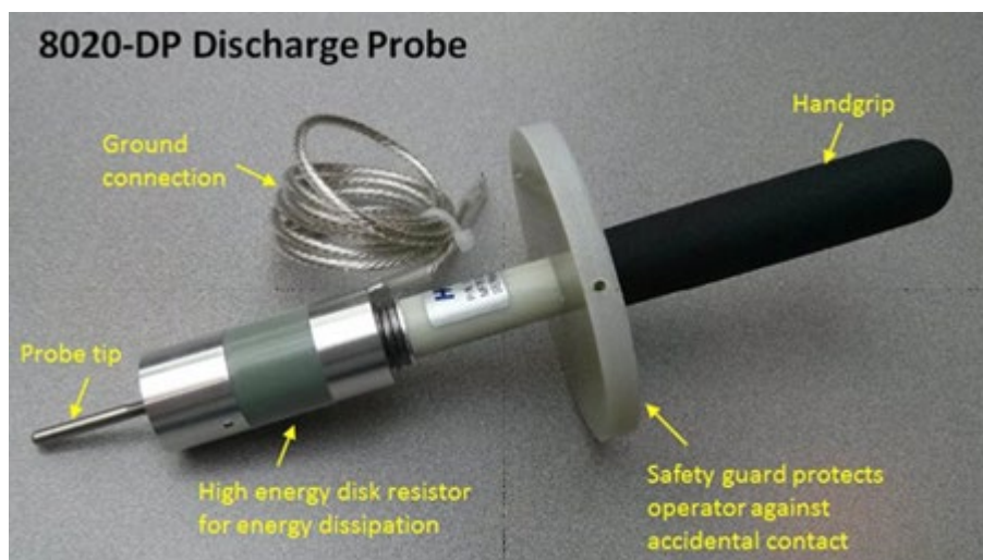
Figure 79: Model 8020-DP High Voltage Discharge Probe
