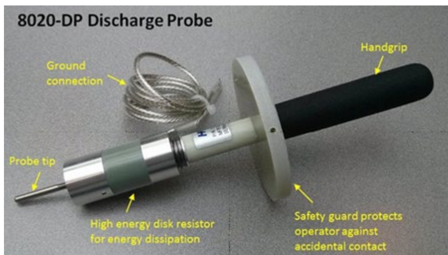
Figure 73: Model 8020-DP High Voltage Discharge Probe
