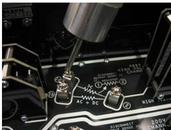
Figure 81: Contacting nodes on the Model 8020 main board
