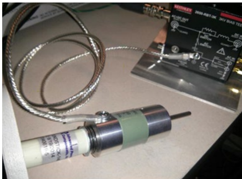
Figure 74: 8020-DP connected to bias tee protective earth screw
