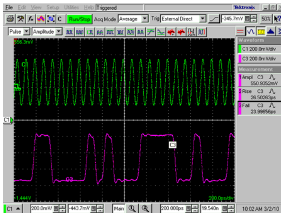
Figure 4: Clock (top) and data (bottom) waveforms
