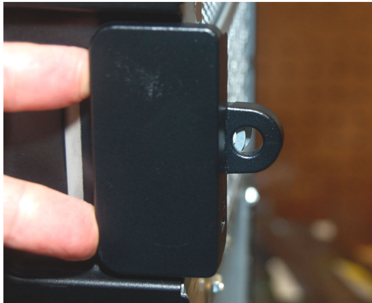
Figure 1: Push the lever back to release the side panel
