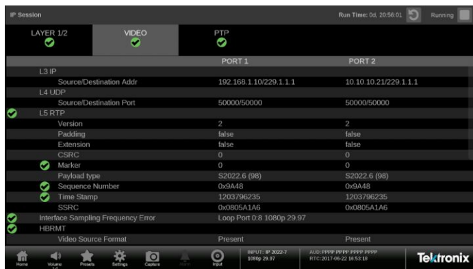
IP Session application showing the RTP header information including HBRMT in ST2022-6 streams in a ST2022-7 configuration.
