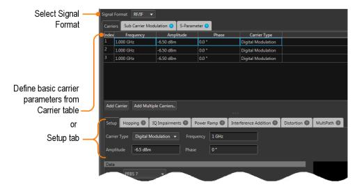
The Parameters shown in the Setup tab reflect the selected (Highlighted).
