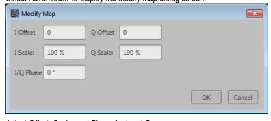
Adjust Offset, Scale, and Phase for I and Q.
