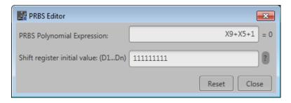
PRBS sequences are generated by a feedback shift register. The number (#) following PRBS indicates the length of the generating shift register. For instance, a shift register with 16 memory cells is required to generate a PRBS 16 sequence. The pseudo-random sequence of a PRBS generator is determined by the number of registers and the feedback.
