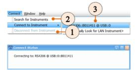
A Connect Status dialog box will appear to confirm the instrument is connected and SignalVu-PC can receive live data from the instrument.
