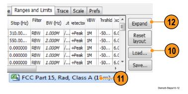
You can edit the start and stop range, filter shape, RBW, VBW, detector, threshold and excursion, and limit line.
