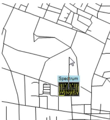
The RSA Map measurement thumbnail display shows the direction of the arrow as you draw it. This display shows the True Azimuth and Magnetic Azimuth. As you change the direction of the arrow, the angles shown in the thumbnail display are updated to help you set the direction accurately. The information shown depends on the map type (geo-referenced or image). The example shown is for a geo-referenced map.
