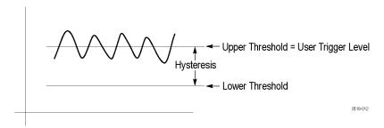
The following figure shows that a trigger is generated when the signal frequency changes sufficiently to exceed the hysteresis value (the difference between the upper and lower thresholds) and cross the lower threshold followed by crossing the upper threshold.
