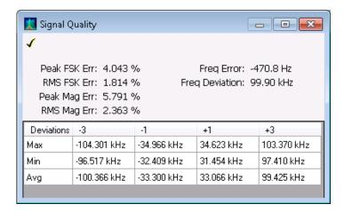
Signal Quality display for nFSK modulation type
