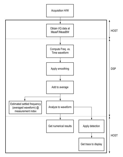
Frequency settling time flow diagram
