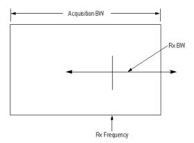
**Case 2.** In this case, the upper and lower limits of the Receiver BW exceed the upper and lower limits of the acquisition bandwidth. When this occurs, audio demodulation will be disabled and an error message is displayed.
