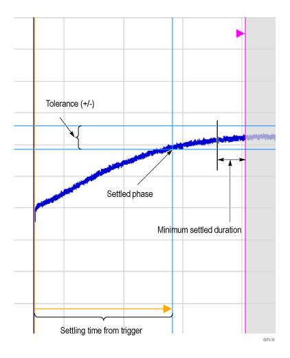
**NOTE.** The blue vertical bar indicating the measurement start time may not appear. Zero phase is referenced to the measured hop, as the phase will not typically have a settled value during the previous hop.
