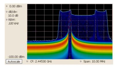
Figure 17. The DPX spectrum display after 5 seconds. The MaxHold trace is cyan.
