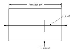
**Case 3.** In this case, the upper and lower limits of the Receiver BW fall within the upper and lower limits of the acquisition bandwidth. This is the desired relationship between the three settings, and audio demodulation is enabled.
