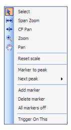
To use the Touch-screen Actions menu, touch the display in a graph area and hold for one second, then remove your finger. You can also use a mouse to display the Touch-screen Action menu by clicking the right mouse button.
