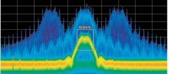
Figure 29. Example of Density Trigger. Left: A free-run DPX display showing pulses with varying frequency. Occasionally, a short pulse in the middle appears for a split instant, but it is hard to capture it with just a Run/Stop button. Right: The triggered DPX displays shows the low-amplitude pulse that was not apparent in the untriggered display. The analyzer was set to trigger whenever the average density in the user-drawn box measured 50% or higher.
