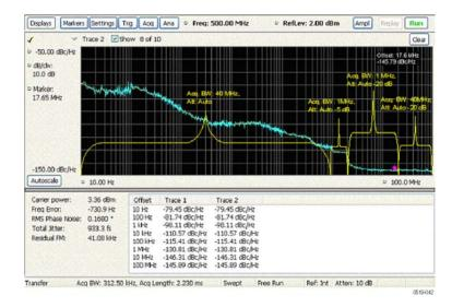
In the previous illustration, the effect of choosing 'optimize dynamic range' is seen. In the offsets between 10 Hz and 1 MHz, the 40 MHz acquisition bandwidth is used, and the RF attenuator is set based on the reference level of the instrument to prevent overload of the RF/IF signal path.
