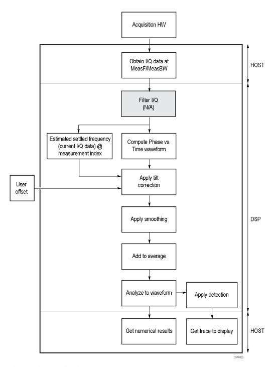
Phase settling time flow diagram
