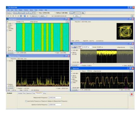
You can drag the Measurement Frequency indicator on the screen to set the measurement frequency. Note the base of the Measurement Frequency indicator. The width of the box indicates the widest measurement bandwidth in use among the open displays. You can see how the width of this box changes with the
