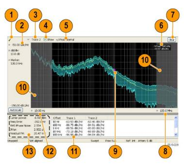
RF Measurements Phase Noise Display
