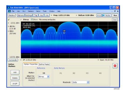
**Searching for peaks on the DPX bitmap trace**. To locate peaks on the DPX Bitmap trace, use the arrow buttons on the Marker toolbar. The left / right arrows move the selected marker to the next peak lower or higher in frequency. The up and down arrows search for peaks at the same frequency. The peaks on the DPX Bitmap trace are defined by the settings for the DPX Signal Density on the Markers > Define Markers > Define Peaks (see page 340) tab.
