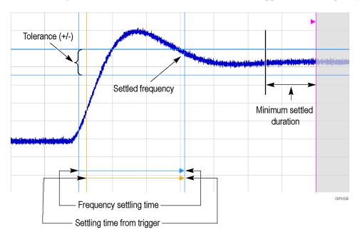
**NOTE.** The blue vertical bar that indicates the end of the previous settled state may not always appear. For frequency settling time, this can happen because the starting frequency is outside the measurement bandwidth.
