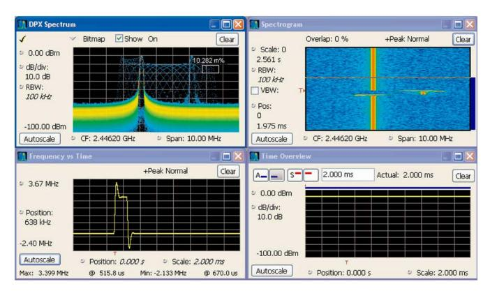
Figure 30. The analyzer triggered when the density in the DPX measurement box exceeded the threshold set by Trigger On This. You can see in the Spectrogram and Frequency-vs-Time displays that the signal event which caused the trigger was a quick frequency hop. The Time Overview shows that the signal amplitude never changed, so a power level trigger would not have worked.
