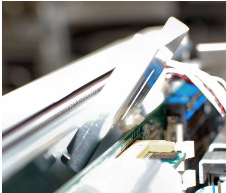
Figure 5: Locating the CPU stopper bracket on the CPU card
