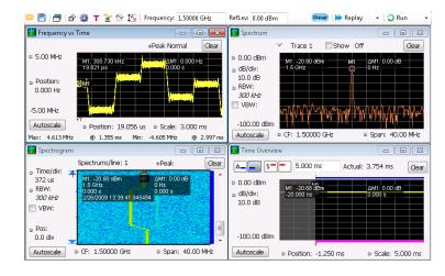
The *Frequency vs Time* display shows the deviation from the center frequency value on the vertical axis and time on the horizontal axis.
