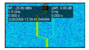
10. Right click the mouse and select Zoom from the resulting menu. Pull the mouse vertically and horizontally to zoom in on one or two hops of the spectrogram signal.
