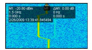
The *Time Overview* display shows log power on the vertical axis and time on the horizontal axis.
