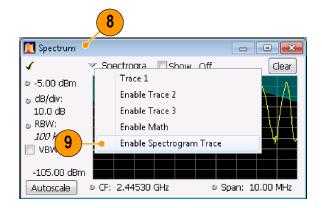
The Spectrogram trace in the Spectrum display corresponds to the line selected in the Spectrogram display by the active marker.
