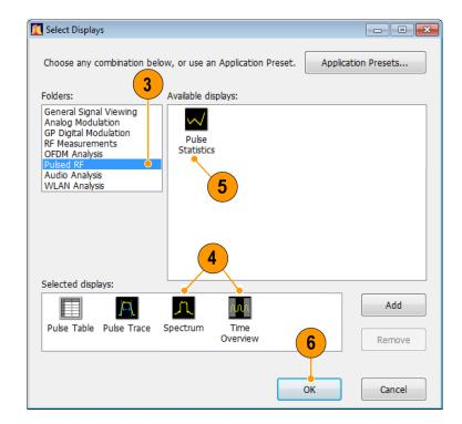
When Trend is the selected plot, the Pulse Statistics display plots the results of the selected measurement for every measured pulse.
